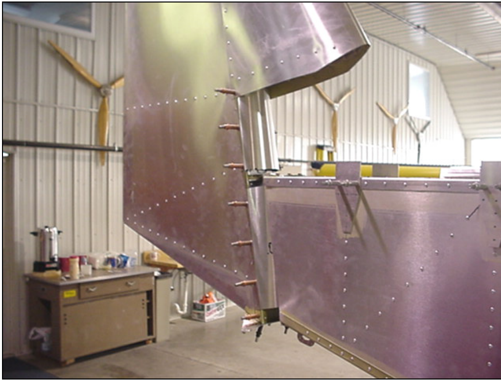
7R3-4 Lower Spar Fairing 7R3-3 Upper Spar Fairing
