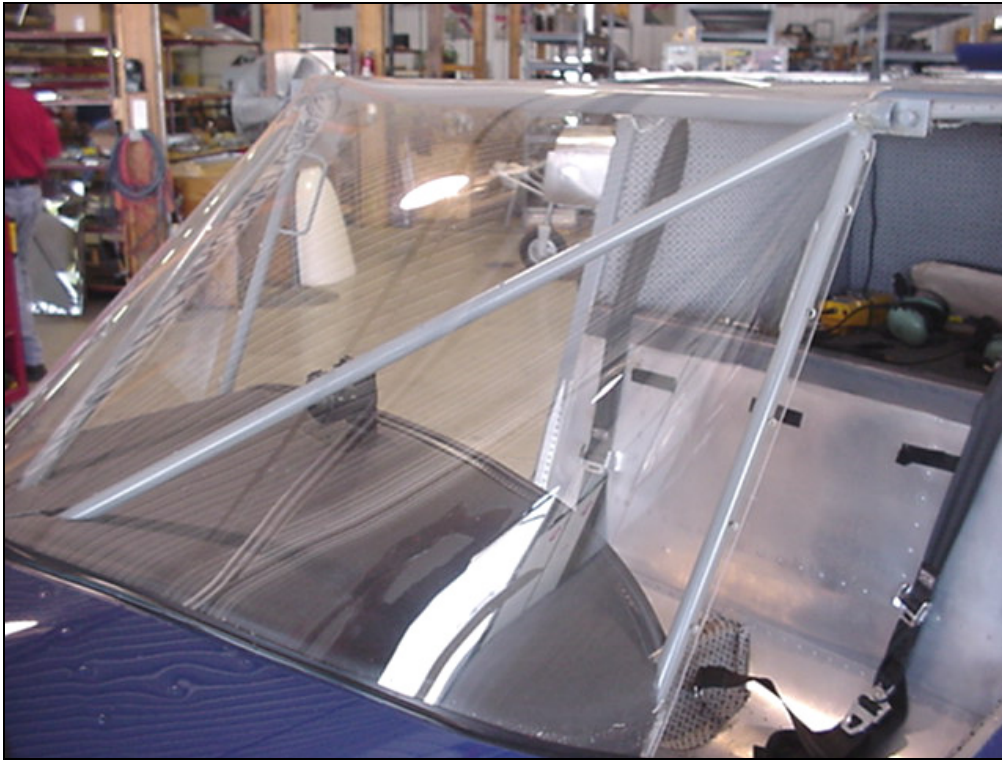
Installation of the Windshield without the wing bolted to the fuselage.
