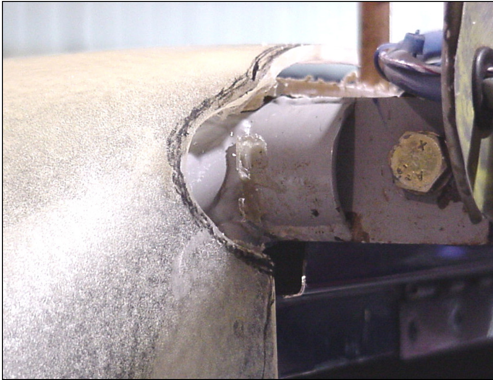
Detail of the Windshield around the main Wing Spar attachment with the Cabin Frame
