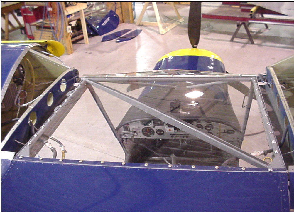
The Windshield can also be installed with the Root Skin 7V9-1 removed
