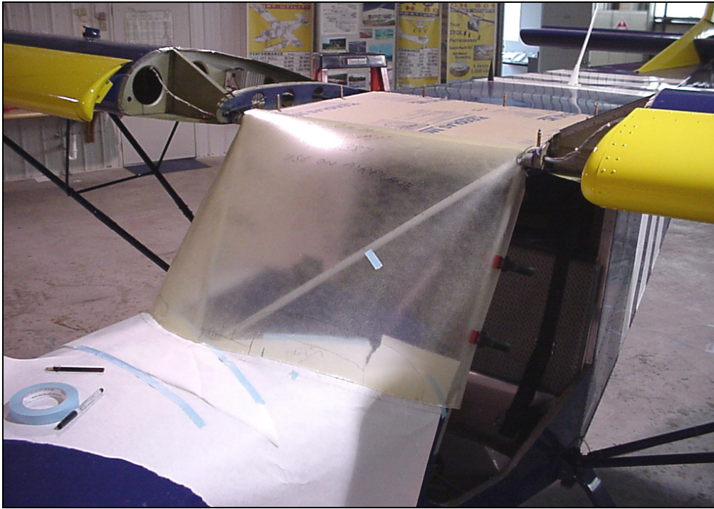
Trial fit of the Windshield to the Fuselage.
