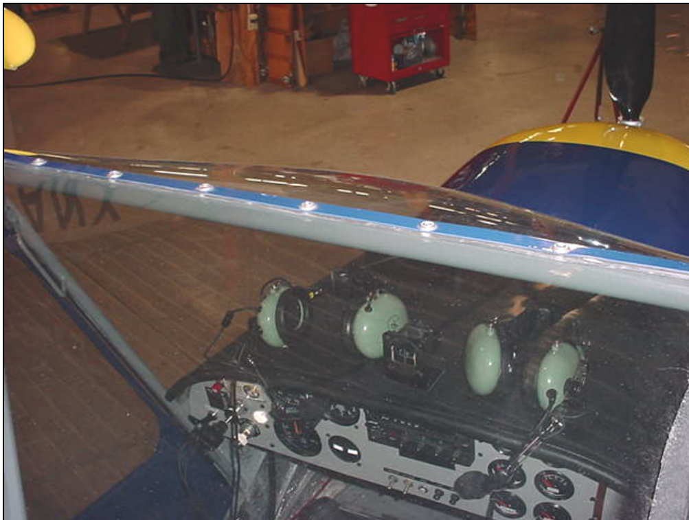
Windshield overlaps on top of the top window 7F19-1
