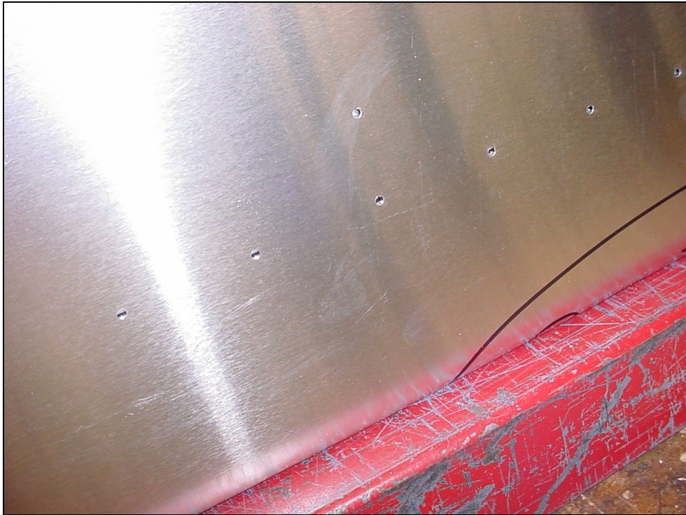
Rivet line visible through the pilot holes.
