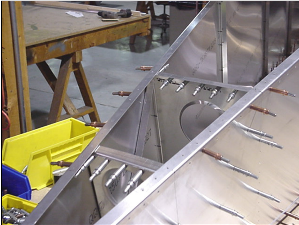
The diagonal and 'L' Angles in position.
