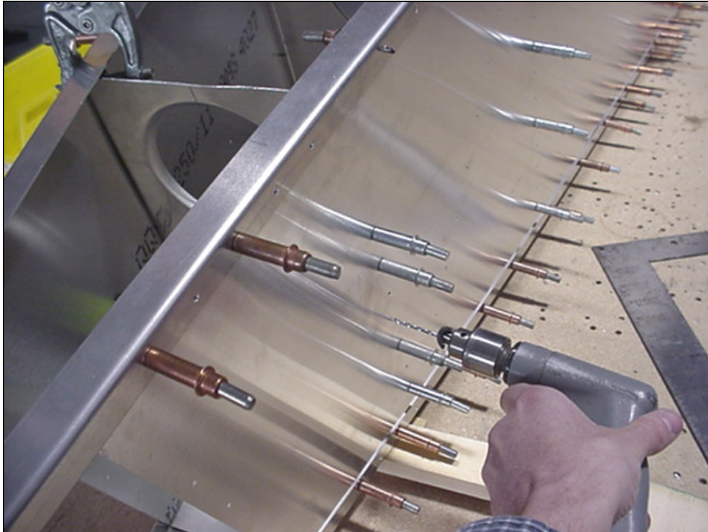
Drill and cleco
