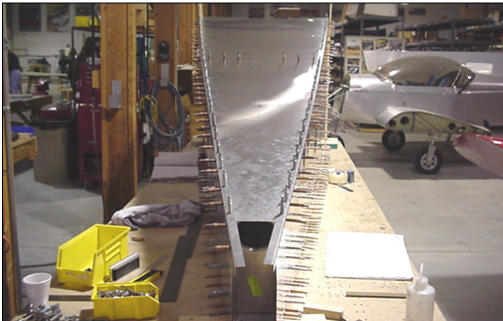
The diagonal and 'L' Angles in position.
