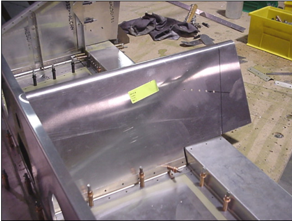
7F11-4 Tunnel 7F11-4A Tunnel Angles
