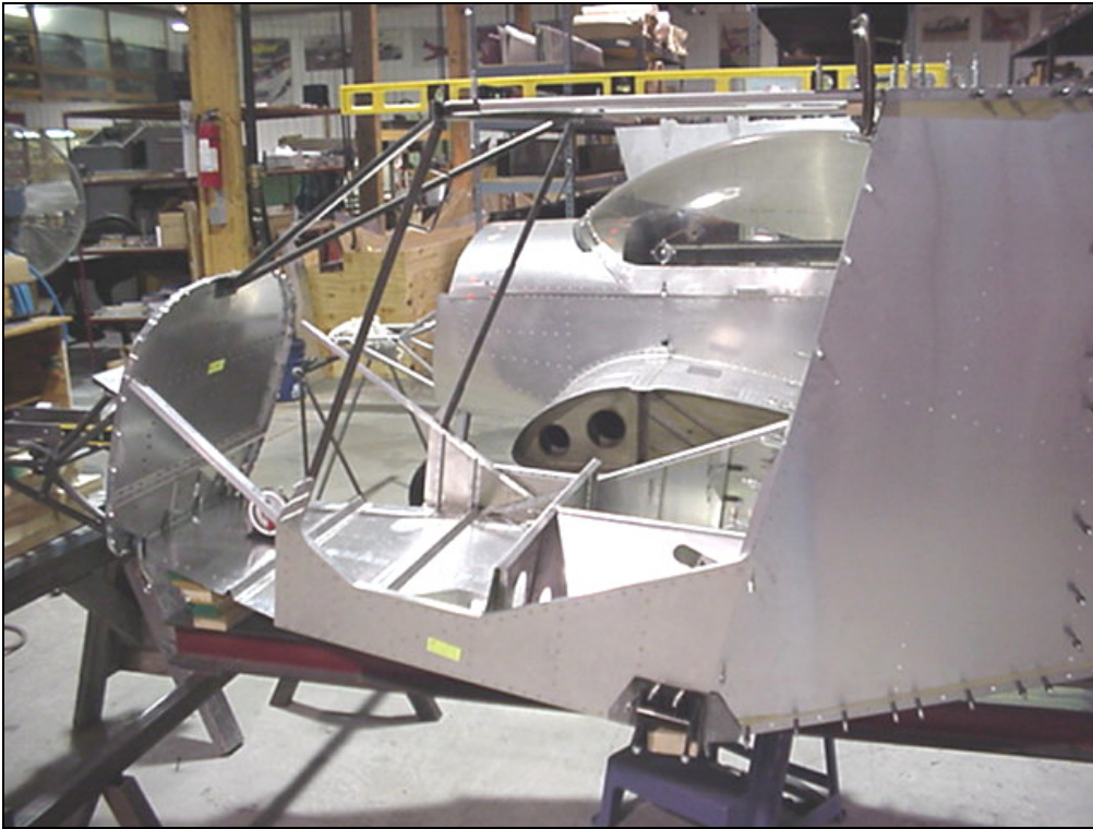
Inside view of right side: The Doubler, 7F3-2, overlaps on the underside of the aft flange of Channel 7F10-1.
