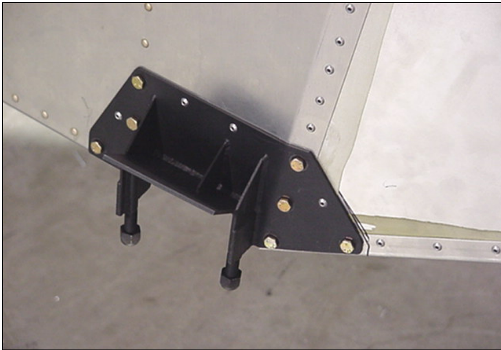
View looking forwards at the left Gear Strut Fitting 7F17-1SP.
