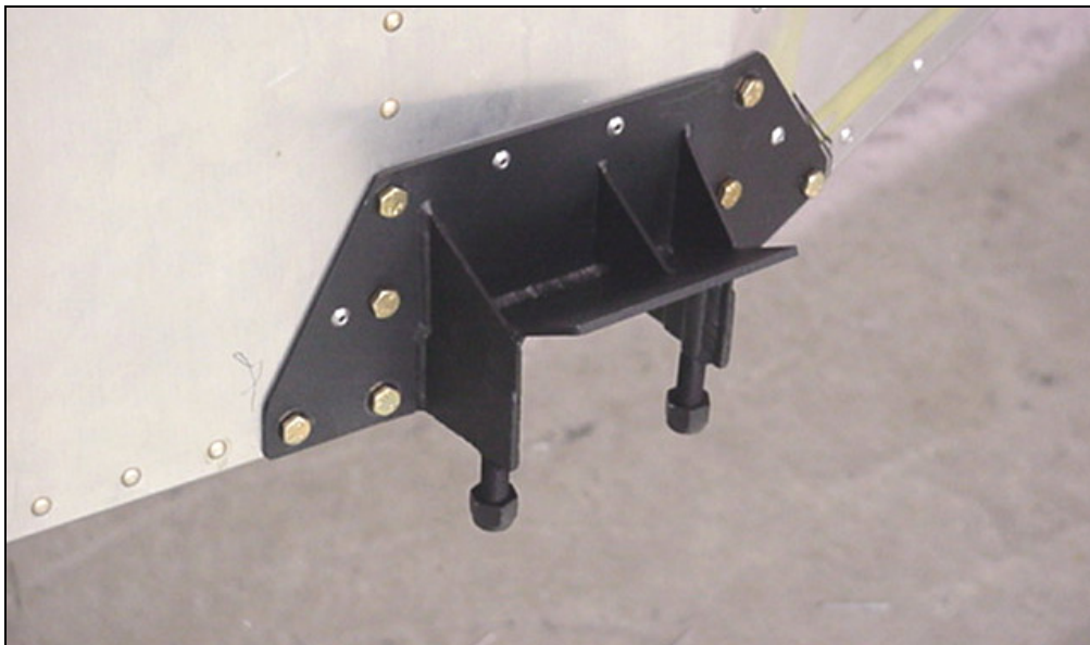
View looking back at the left gear strut fitting 7F17-1SP.
