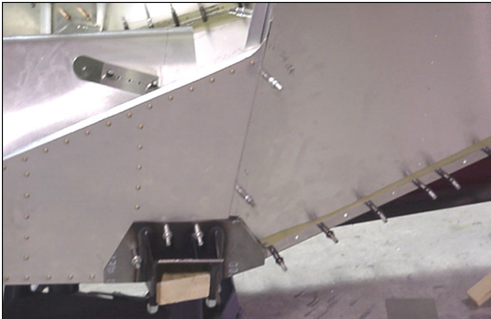
Ref: 7-F-10 The Bottom Longeron Doubler, 7F3-2, and the Bottom Skin, 7F2-2, overlap underneath the aft flange of the Bottom Channel, 7F10-1 (looking up at right side)
