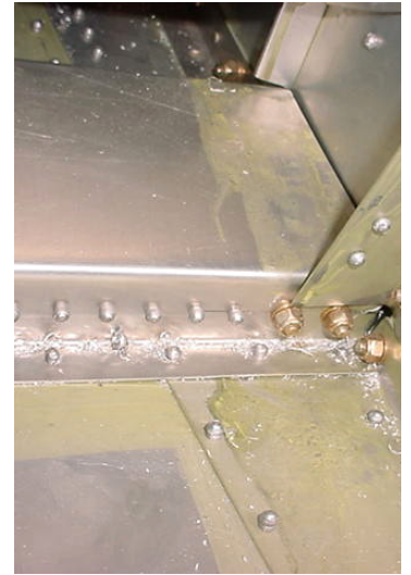
Inside view of right side: The Doubler, 7F3-2, overlaps on the underside of the aft flange of Channel 7F10-1.
