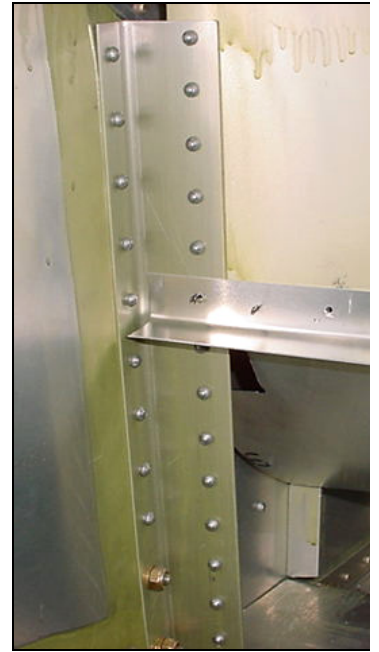
The ends of the 'L' Angle overlap on top of the Upright 7F11-5
