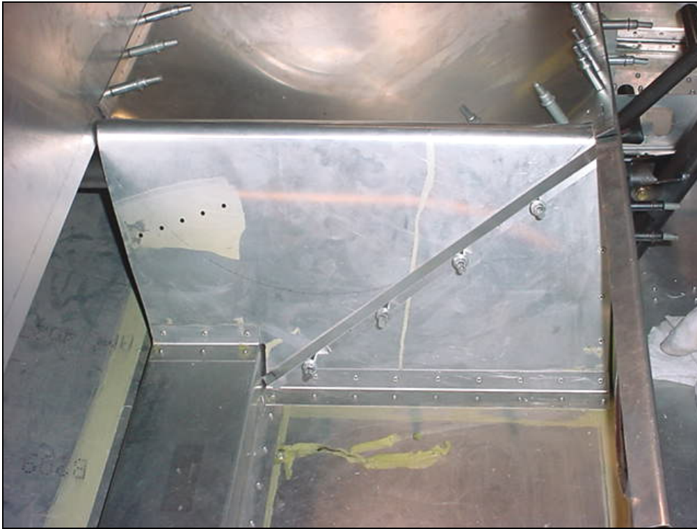
'L' Angle, detail of bottom aft corner Ref: 7-F-16
