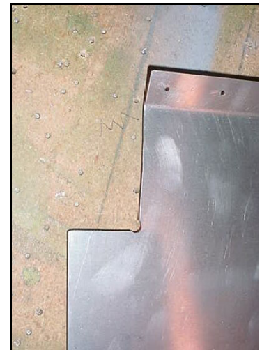
Detail of rear outboard cutout: 75x32mm
