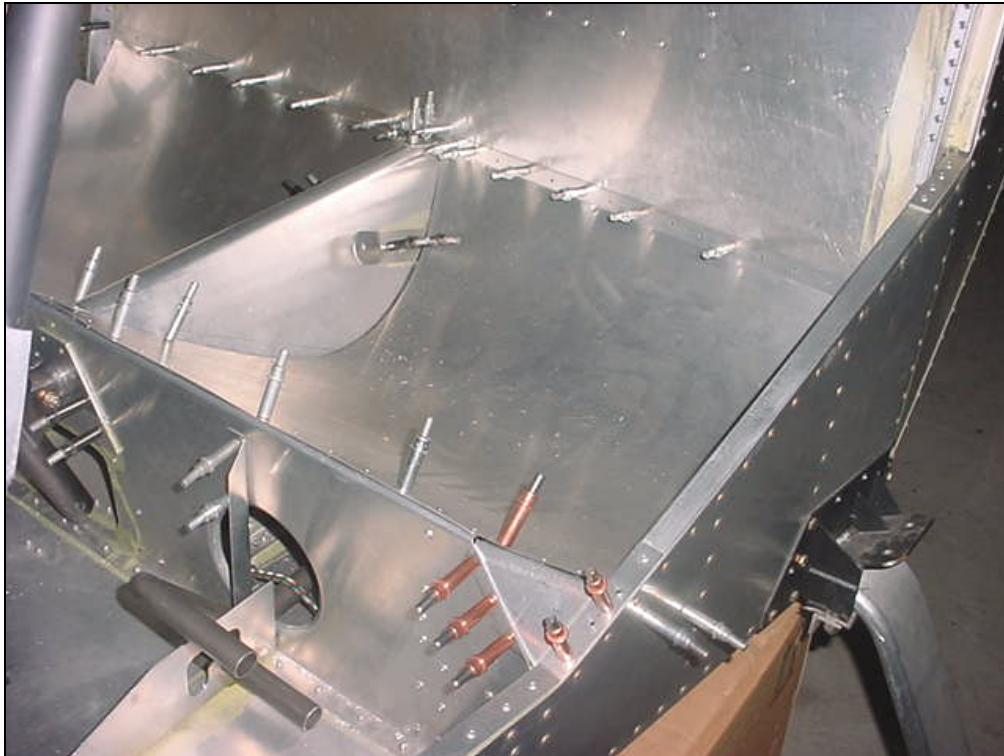
Gusset, left side
