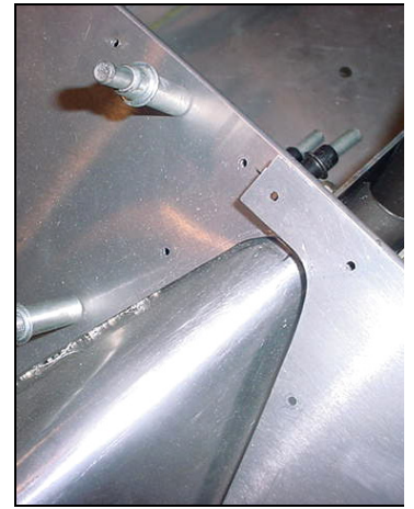
Trial fit template to determine the inboard cutout on the Seat 7F16-1
