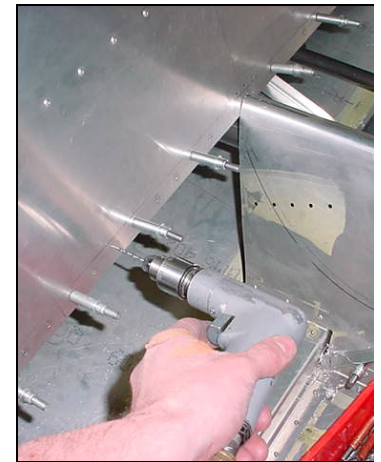
Back drill the 'L' Angle through the hole in the Seat Back (holes for the seat)
