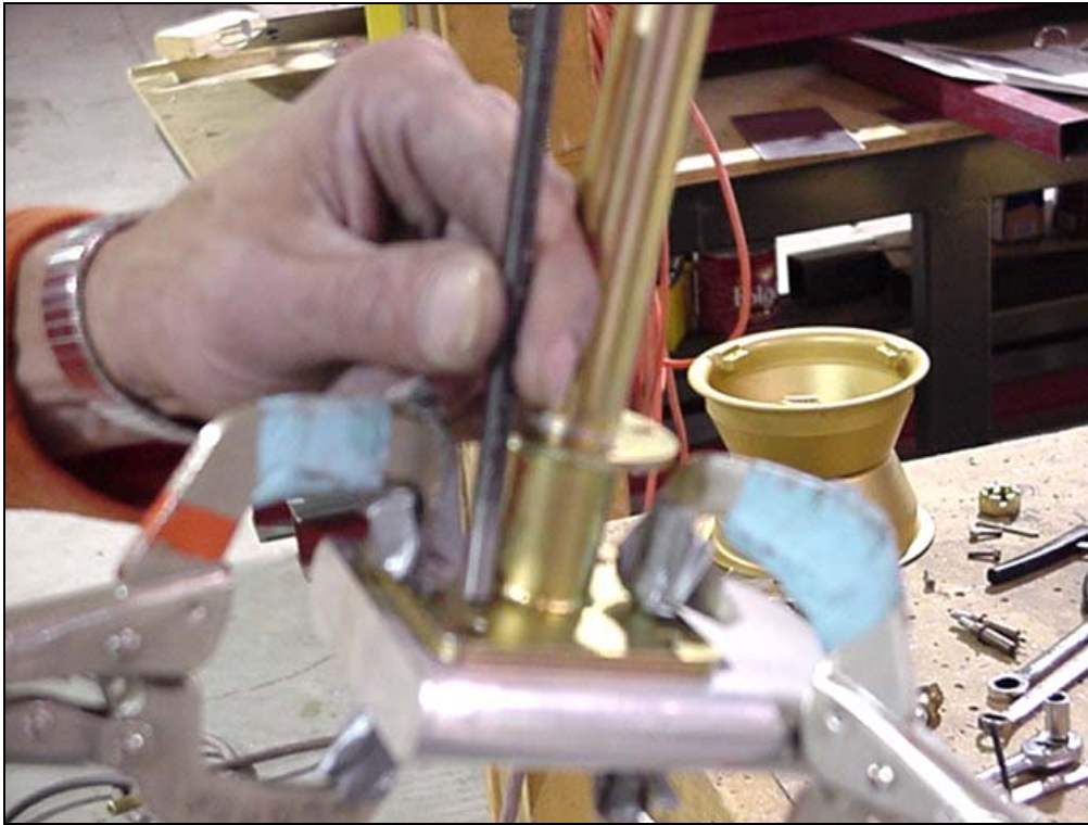
Transfer Punch for drilling the Main Axle to the Gear (1/4").
