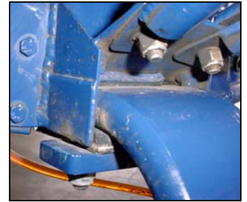
Detail gear strut fitting: The gear is firmly held in place between the top and bottom rubber spacers.
