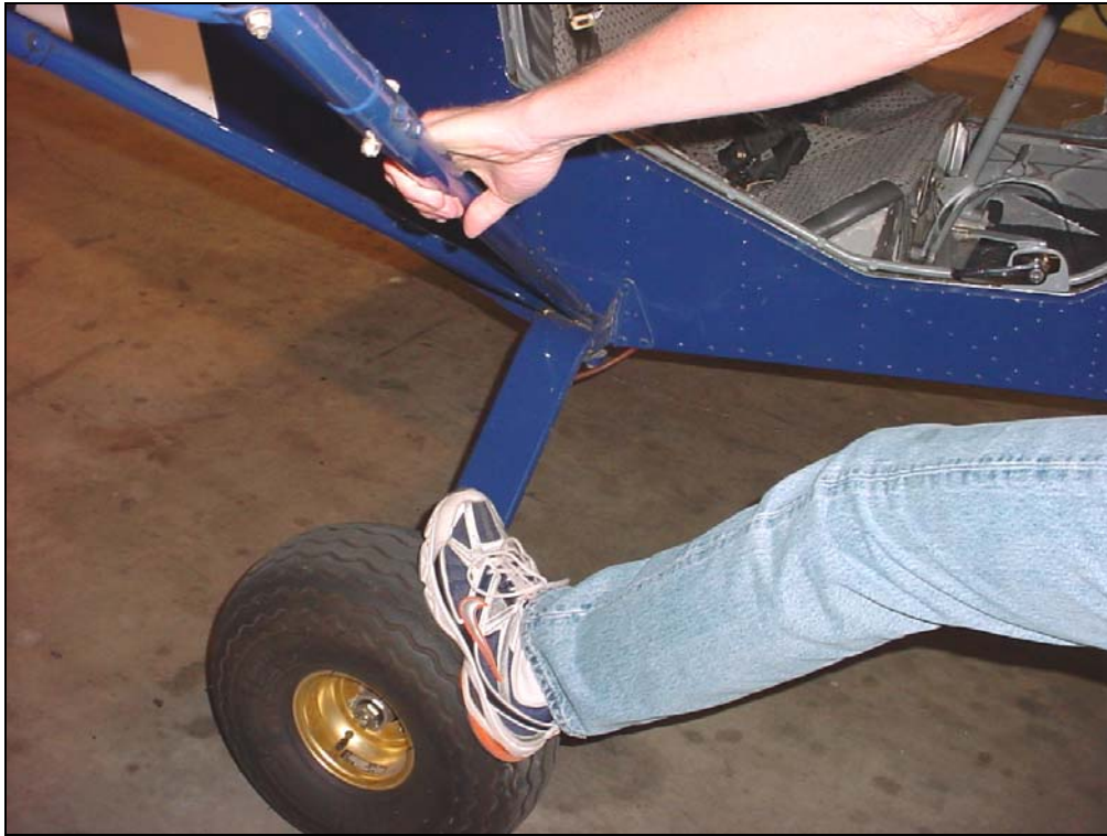
Detail gear strut fitting: The gear is firmly held in place between the top and bottom rubber spacers.
