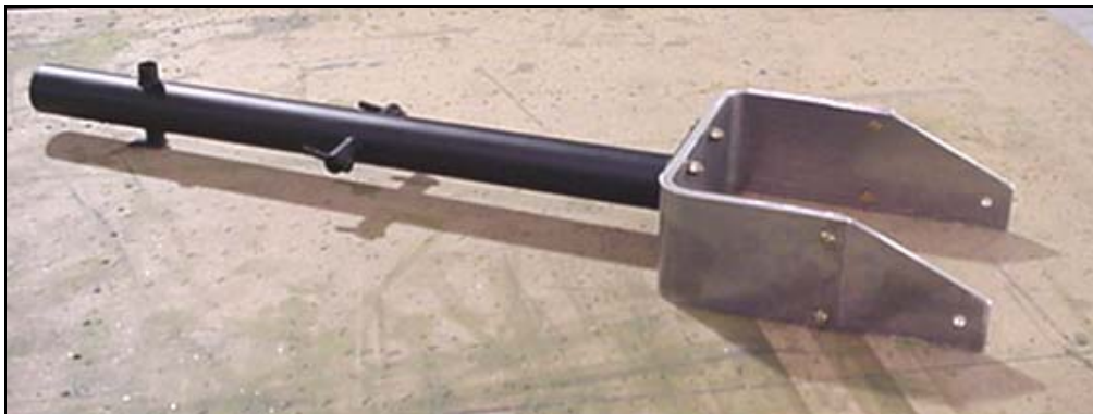
7L12-4J Nose Wheel Fork 7L2-3J Wheel Fork Doubler 7L1-1J Nose Gear Strut Assembly
