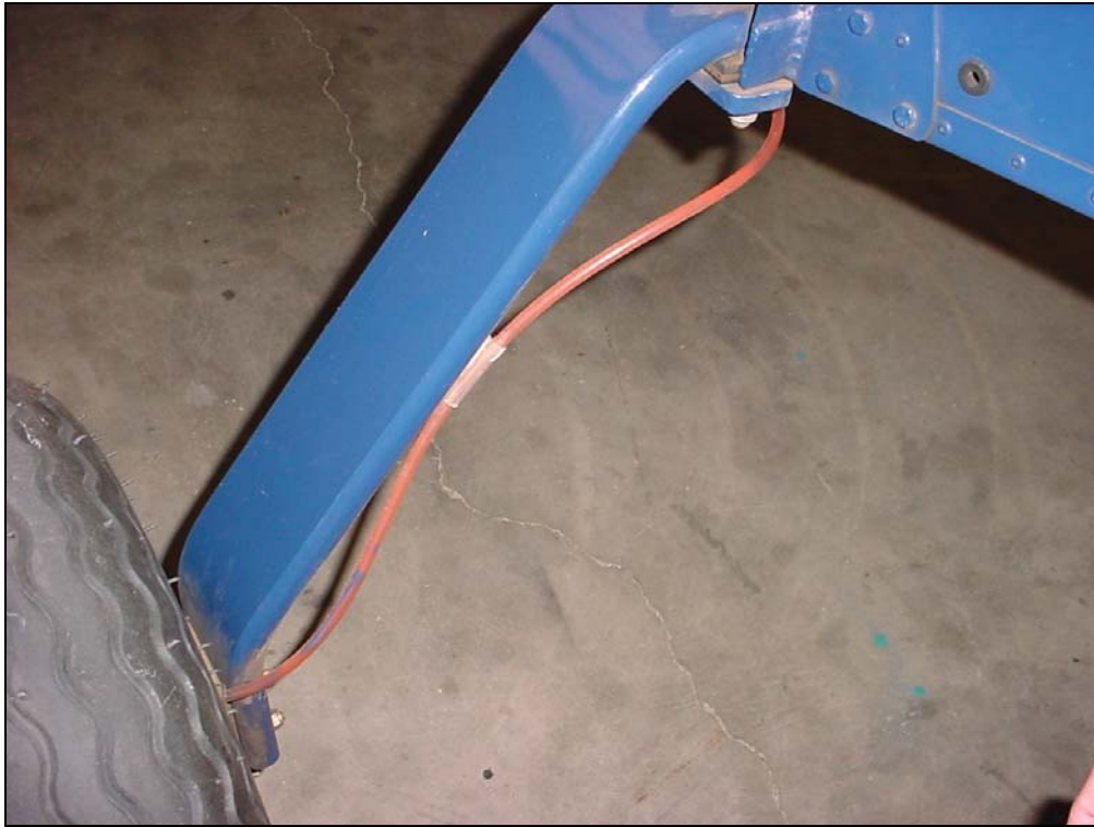
Looking down at the back side of the gear (left wheel). Plastic clip to hold brake line:
