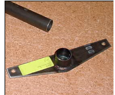
Drill the two 5/16" hole for the Bolt AN5.
