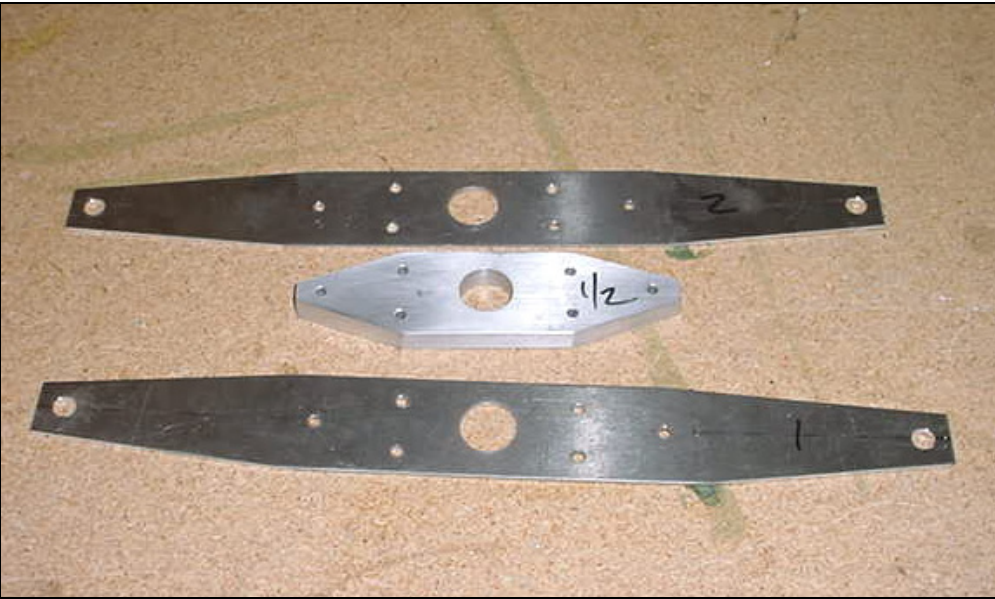
Part after they have been cut, drilled and deburred
