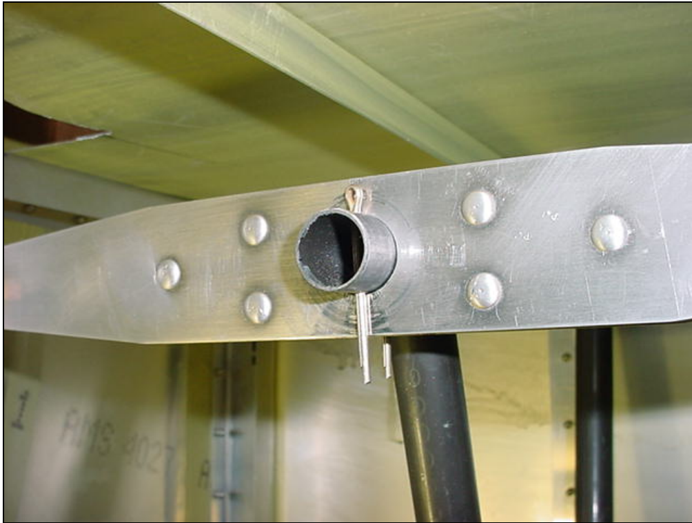
Photo shows cotter pin on the aft side of the Flaperon Bellcrank.
