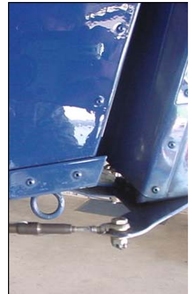
Rudder Horn 7R2-3, the legs are bent down
