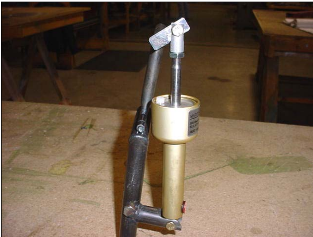
Cutout in 3/4" tube for the lower attachment
