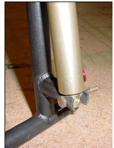
Cutout in 3/4" tube for the lower attachment
