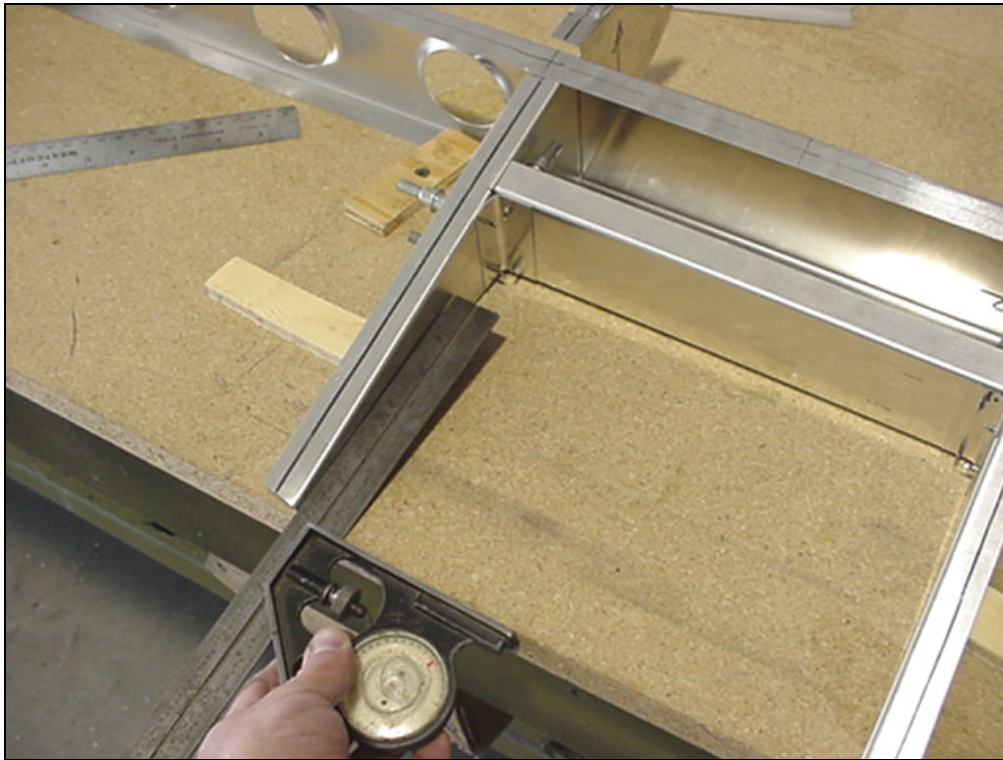
7H2-9 Elevator Channel
