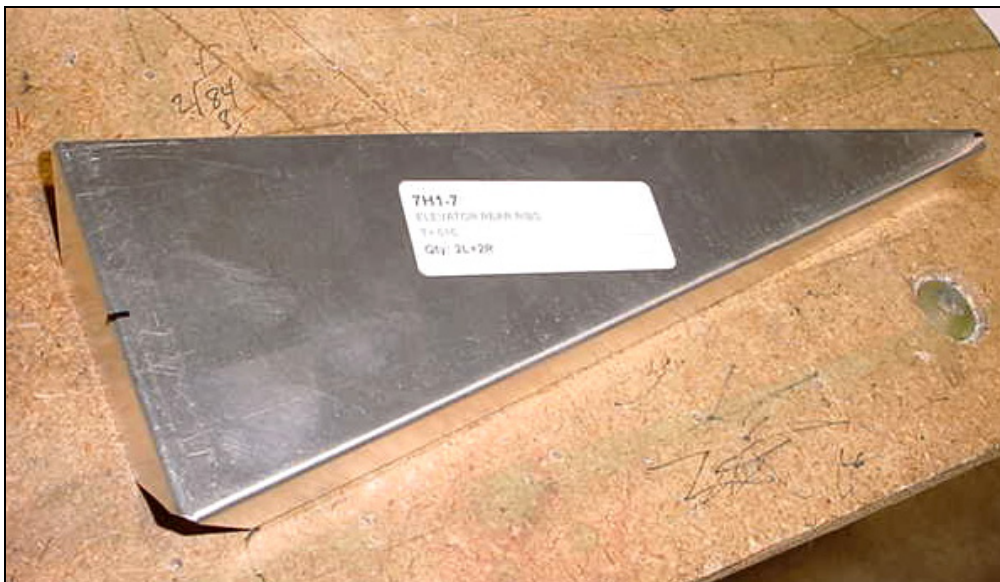
ELEVATOR REAR RIBS 7H1-7
