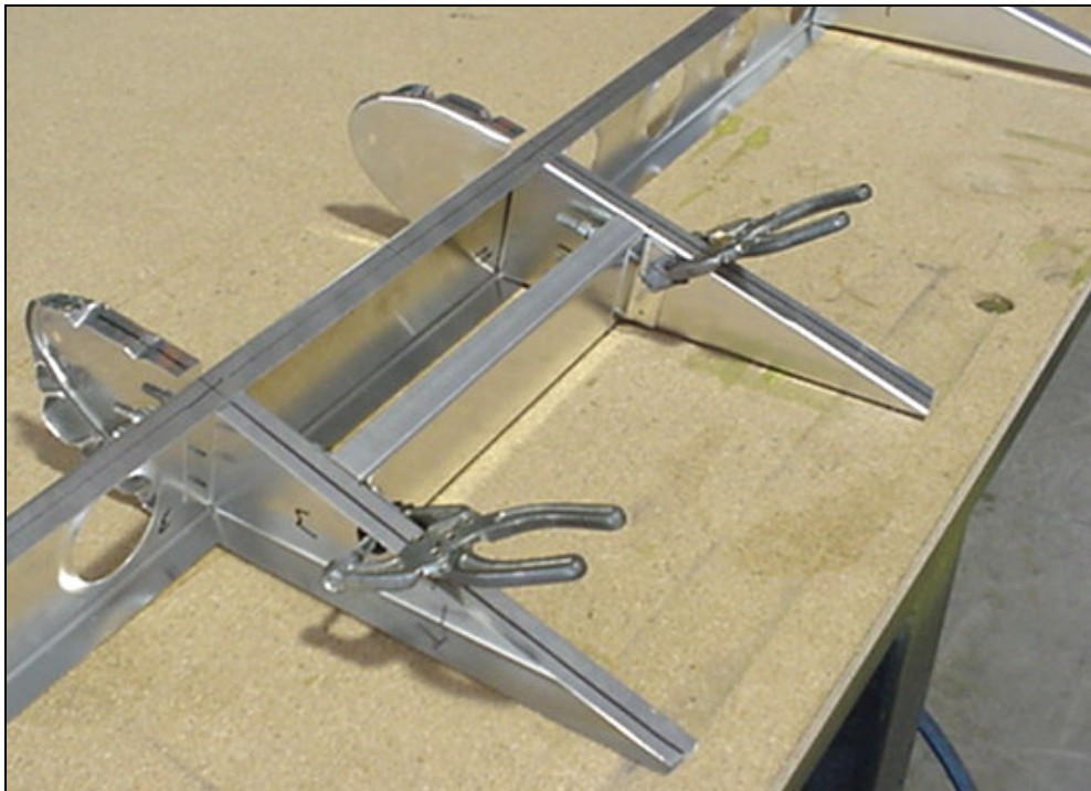
7H2-6 Elevator Channel
