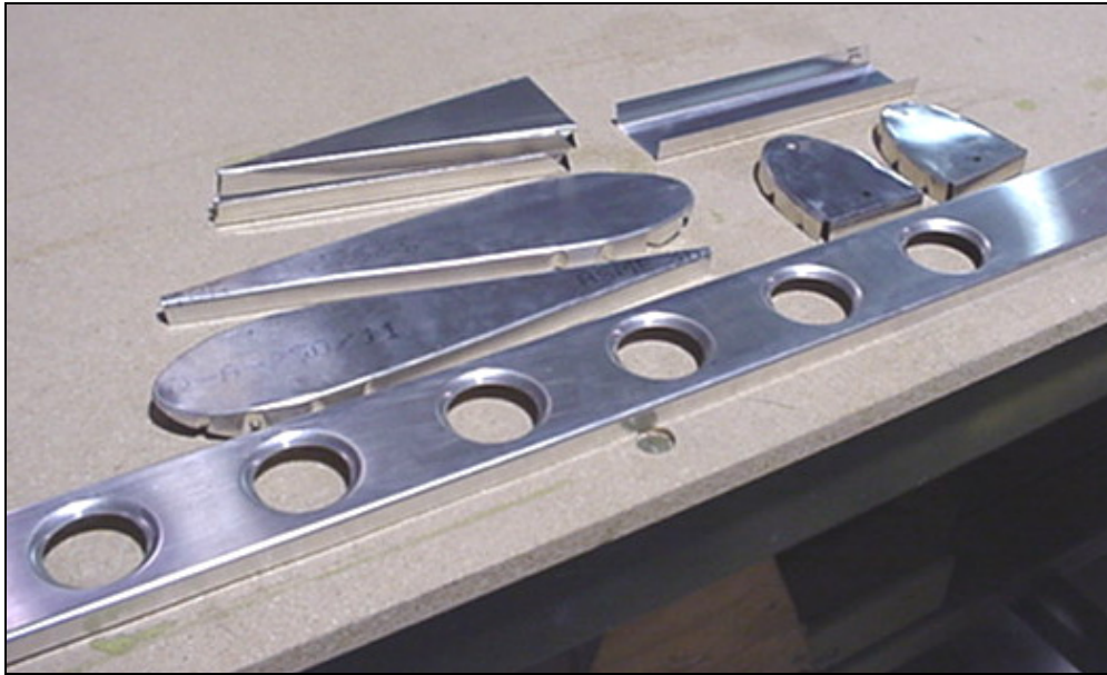
The elevator skeleton parts.
