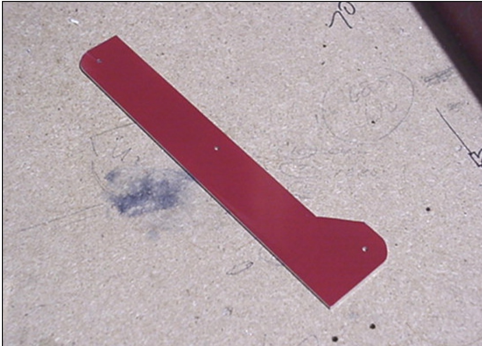
Elevator Horn Cable Holes Positioning Template
