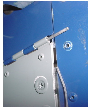
Detail of top rear corner of left door. Aft edge of the bubble door is tapered back to make it easier to install the pin through the piano hinge.
