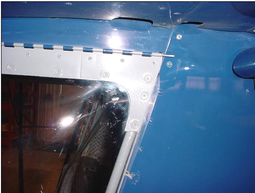
Detail of top rear corner of left door. Aft edge of the bubble door is tapered back to make it easier to install the pin through the piano hinge.
