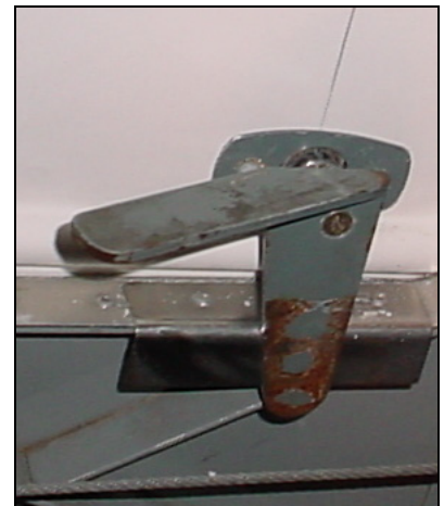
Inside handle in closed position.
