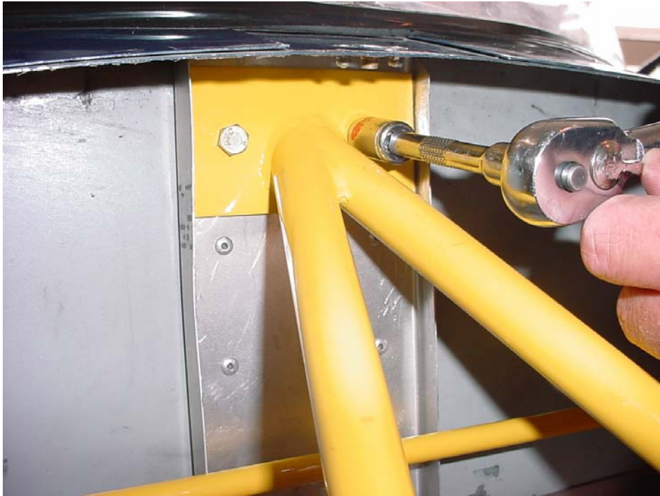
The upper holes are drilled through the firewall and into the cabin frame 7F18-1.
