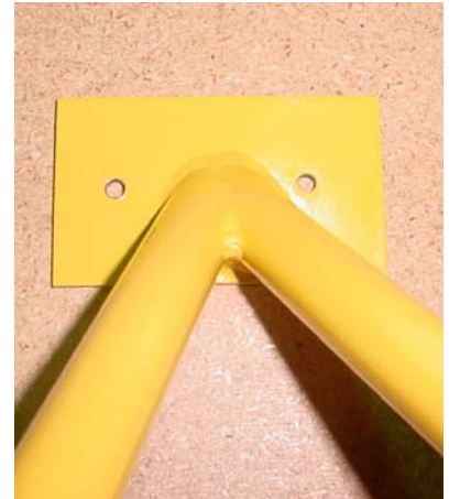
The upper holes are drilled through the firewall and into the cabin frame 7F18-1.
