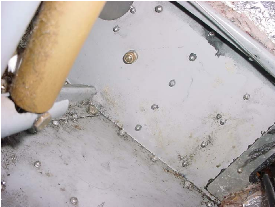
AN3-5A Cabin side of firewall, lower engine mount bolted to firewall.
