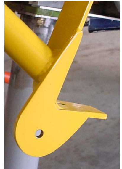
Float fitting welded to the side of the lower bracket.
