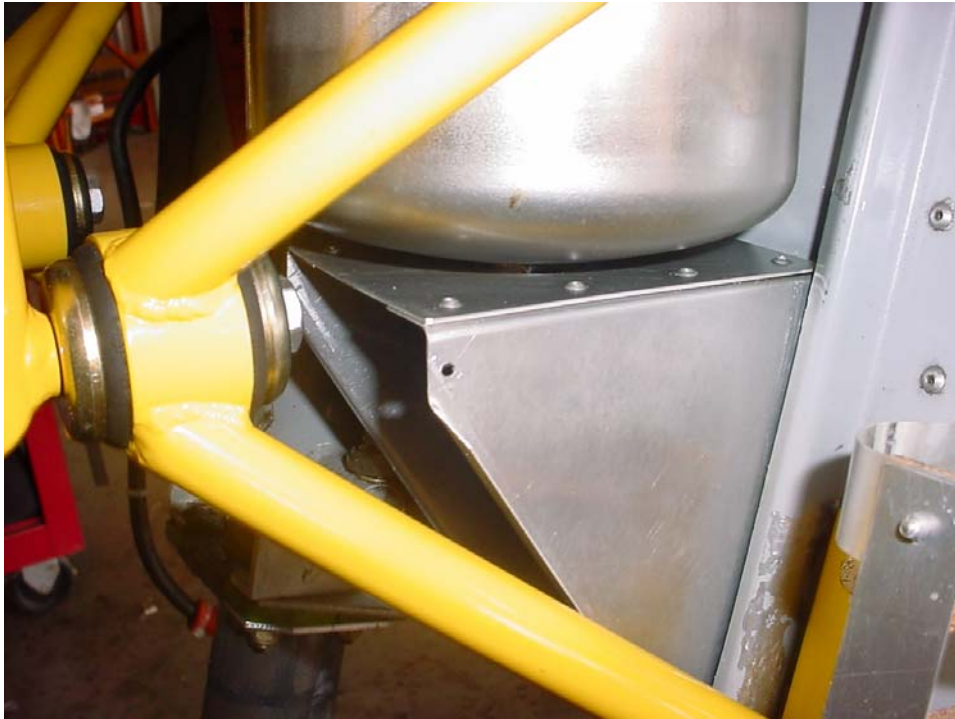
4 rivets 4A top plate to side bracket.
