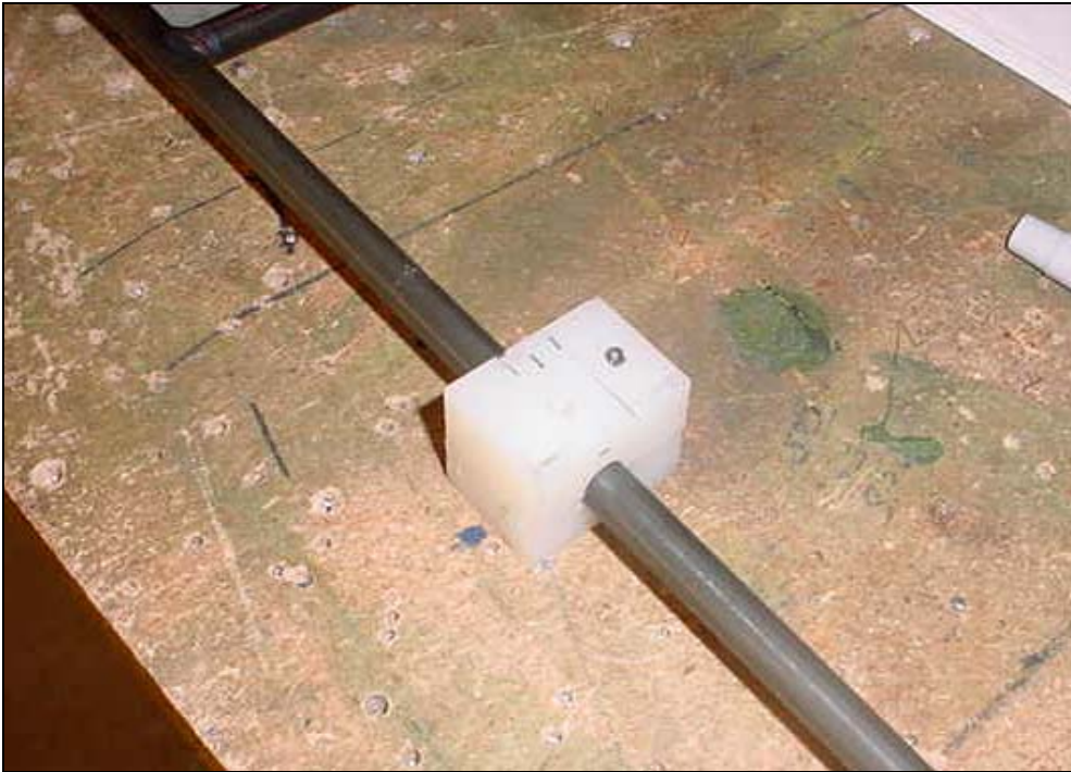
Location of the 3/16" hole Edge distance = 8mm.
