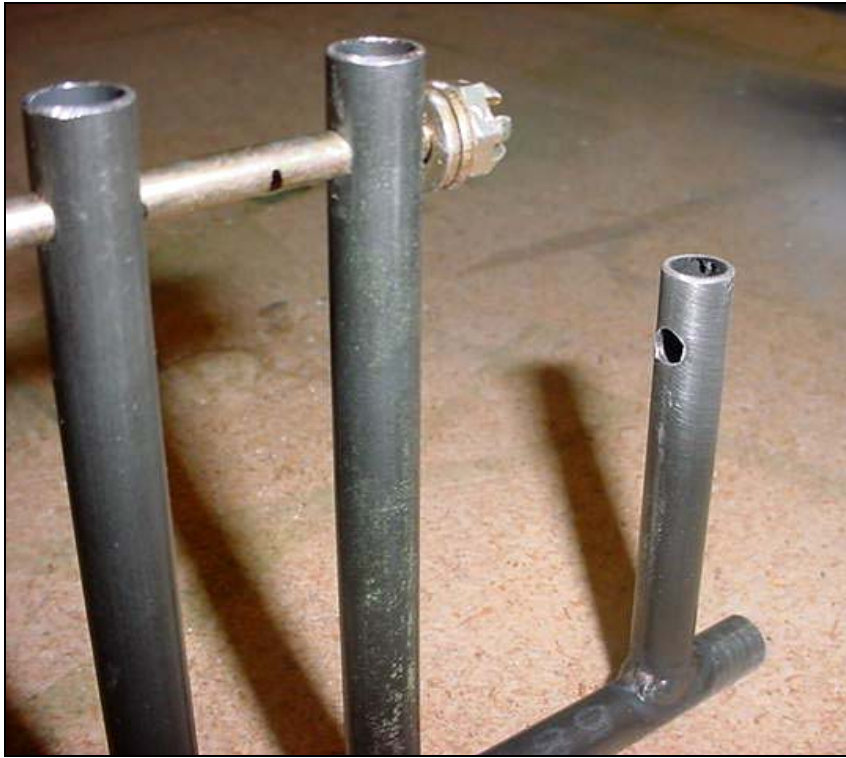
3/16" hole for the Throttle Rods 7E5-4 in the left and right vertical tube on the Bell Crank 7E5-1
