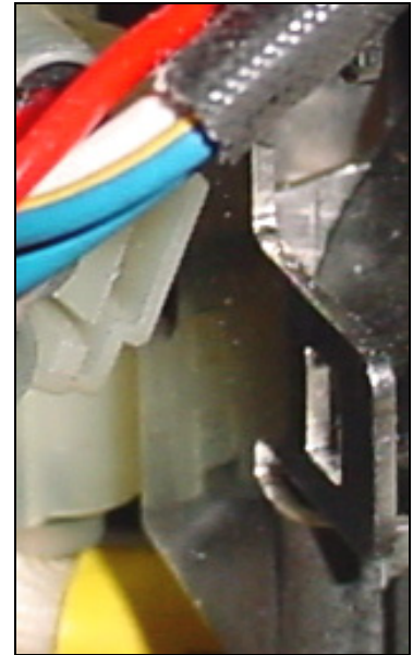
Square hole in steel mounting bracket.
