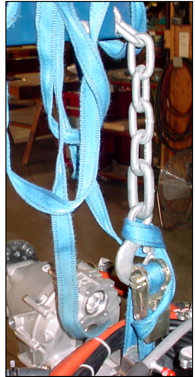
Strap across the steel bracket to the chain.
