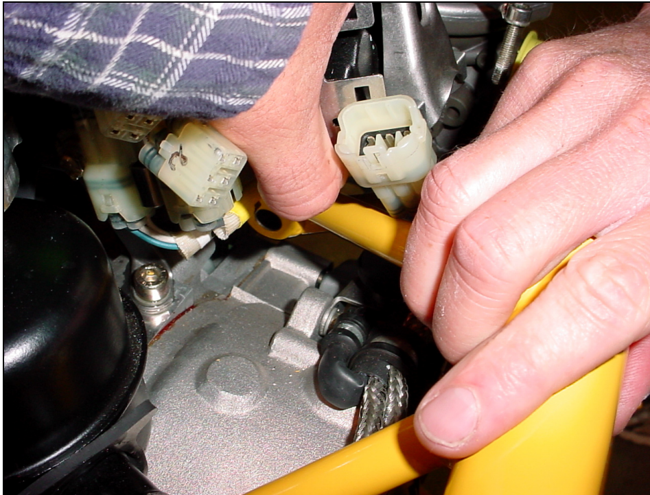
Lift up on the coils to work the ring mount over the top of the mounting bracket.
