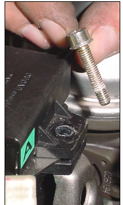
Holding the screw by the ring connector.
