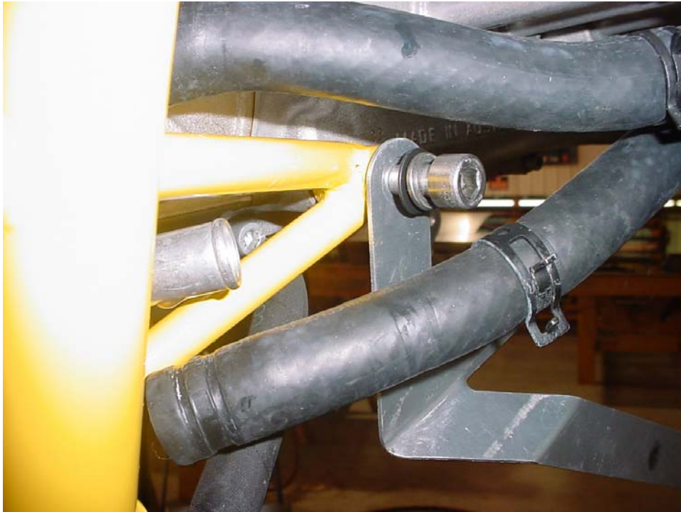
Rear right bolt. 15.5mm spacer fits inside engine mount recessed hole.
