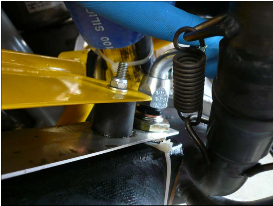
Press on the oil line. Left attachment of the Oil Cooler.
