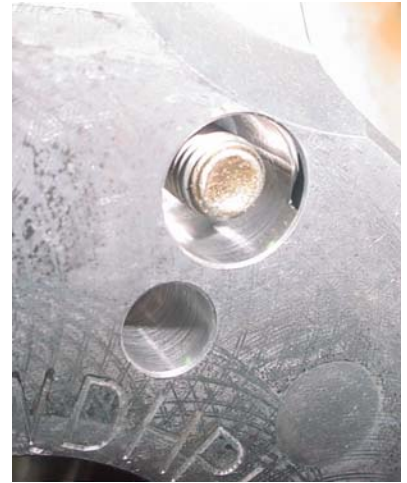
Note: recess for pressed threaded fitting on engine propeller flange.
