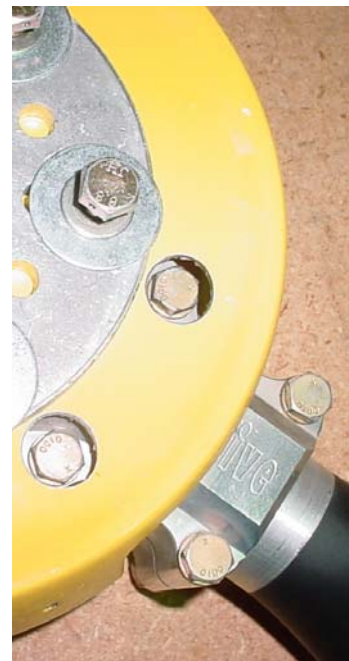
Note: Use large thrust washer along with flat washer on propeller bolts.
