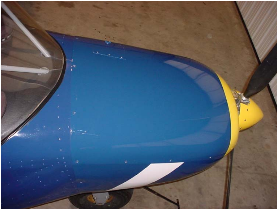
Aft edge of cowl is not parallel to the firewall rivet line.
