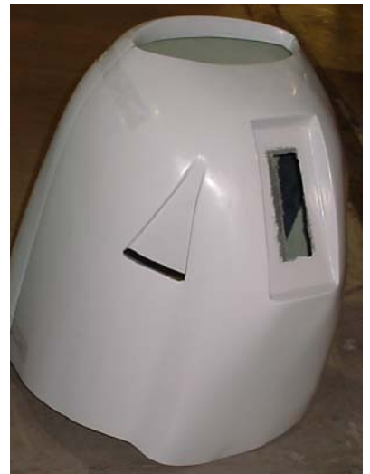
Bottom cowl is not supplied with the cutout for the nose gear leg.
