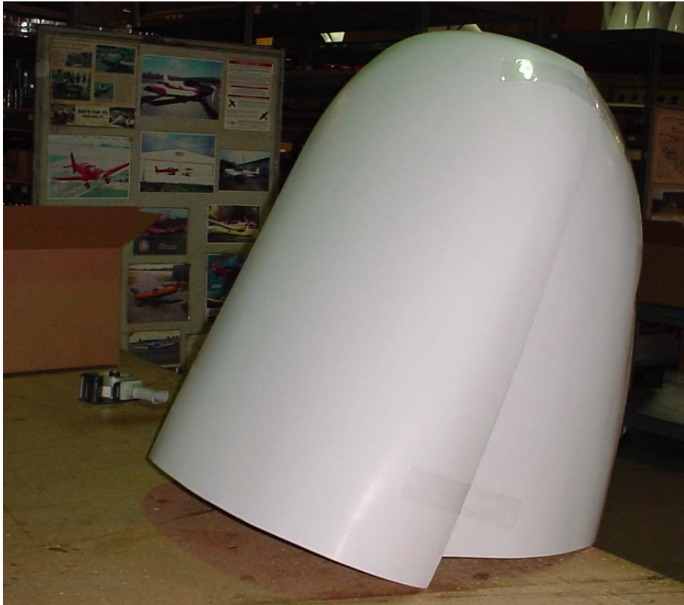
Edge of supplied cowl is oversize. It must be trimmed to fit the aircraft.
