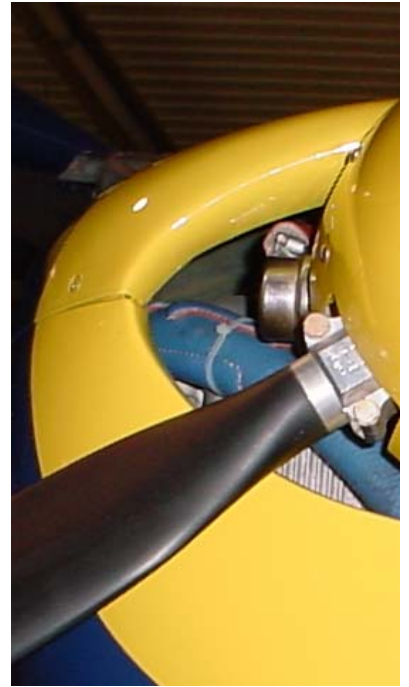
Spinner is centered left and right on cowl opening.
