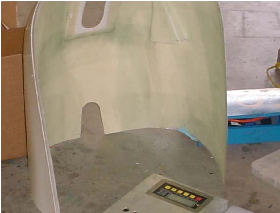
Trial fit of bottom cowl. Cutout for nose gear leg.
