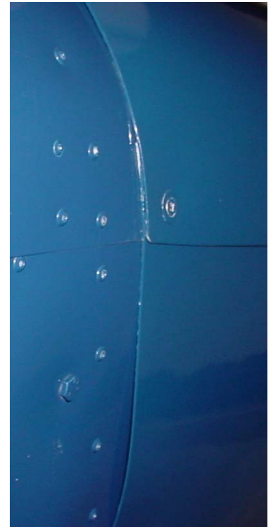
Screw through the top, bottom cowl into the forward top skin and forward fuselage skin.
