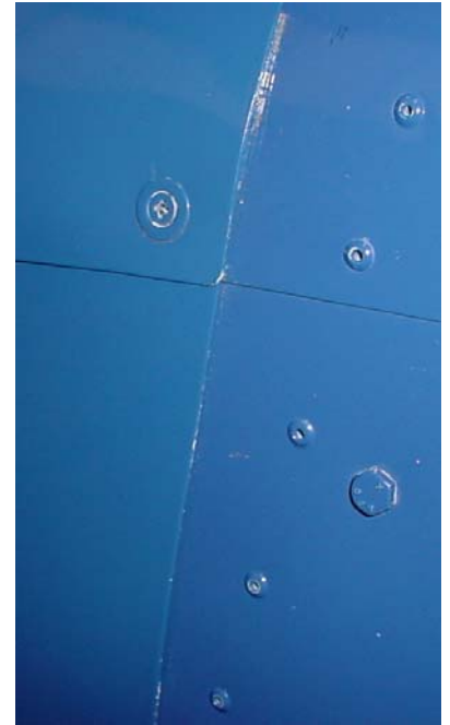
The bottom edge of the top cowl is even with the bottom edge of the forward top skin.
