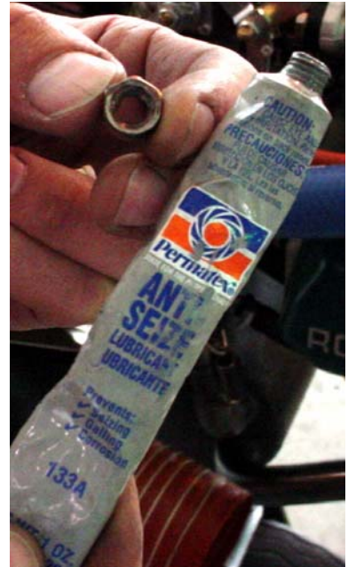
Install nuts for elbows with Anti-Seize.
