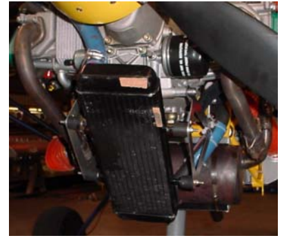
Front view of the radiator between the left and right front elbows.
