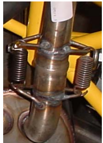
DETAIL: Spring holding the ball joint together on rear elbow.
