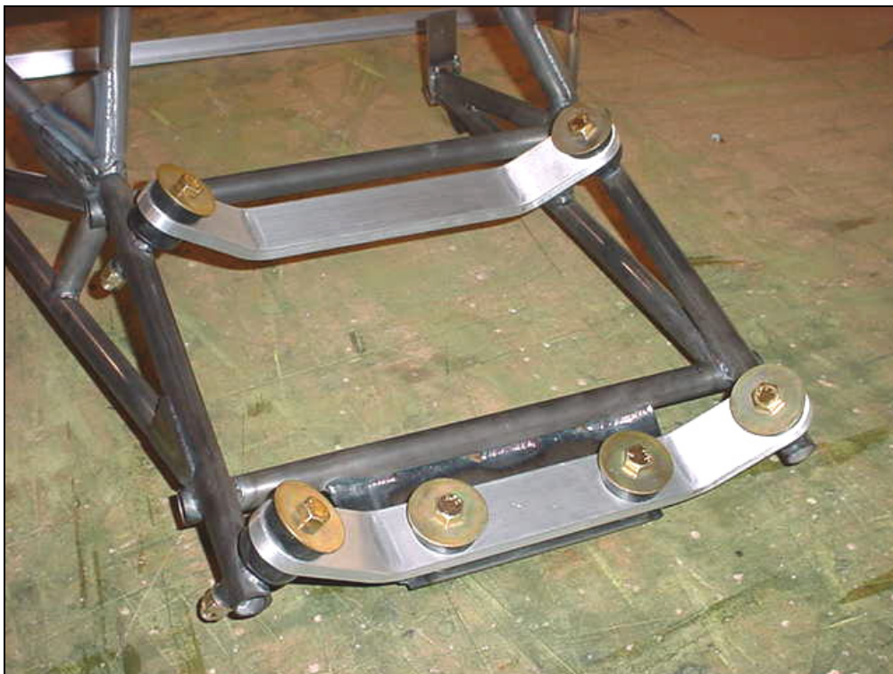
Detail of the Barry mounts at the front of the engine mount: between the "tray" and the front Bracket E2-1X
