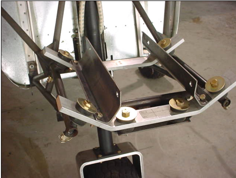
Detail of the Barry mount between the engine mount and the Dynafocal bracket E2-1X Qty = 4
