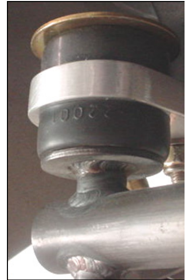
Detail of the Barry mount between the engine mount and the Dynafocal bracket E2-1X Qty = 4
