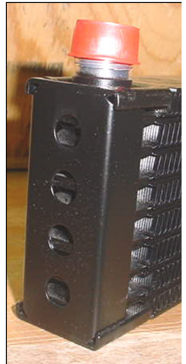
Rotax oil cooler 886-027 Size: 82mm 3.32"
