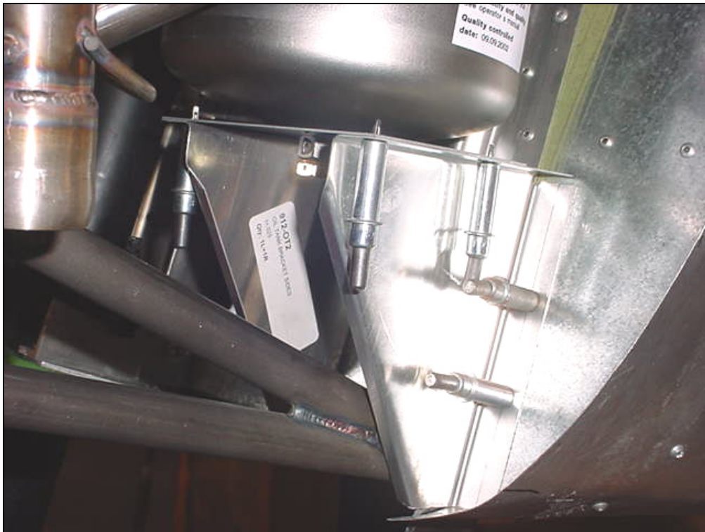
4 RIVETS A4 7E3-2R into 7F1-1
