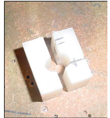
3/8" hole through both blocks
