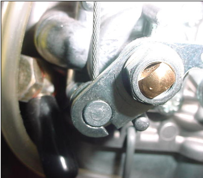
Left Carb: the mark on the choke shaft points towards the cable engagement.
