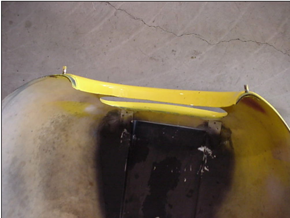
Cowl pins installed on the inside of the bottom cowl
