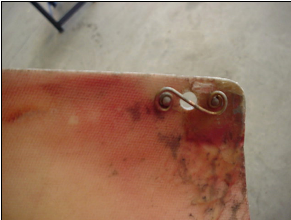
Detail of Dzus on the backside of the top cowl.
