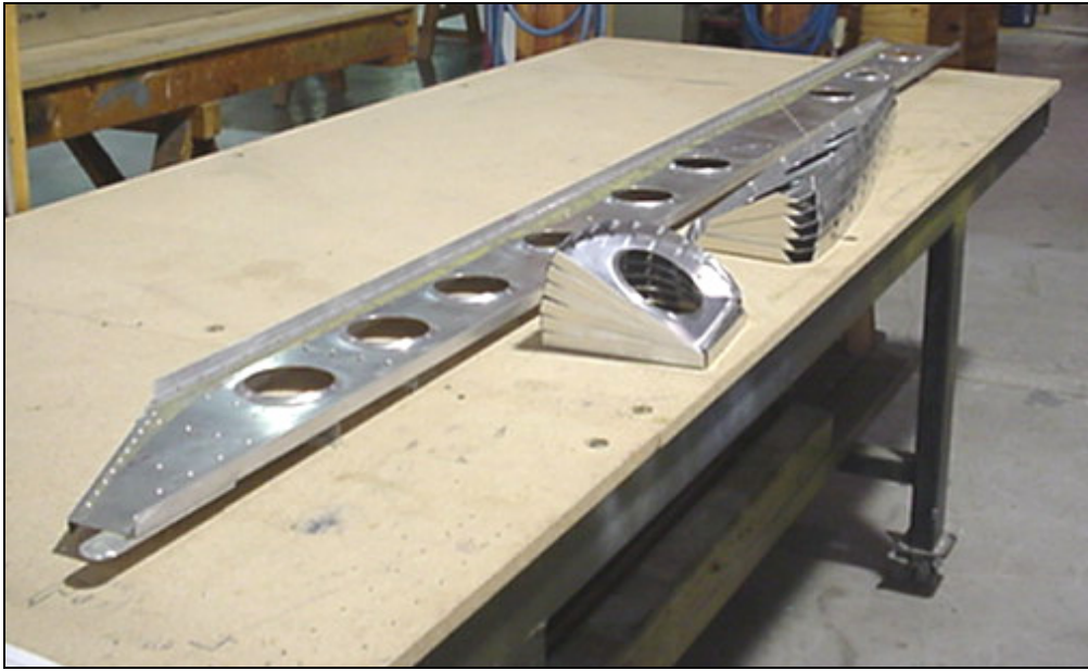
Assembly of the right wing skeleton.
