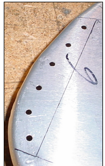
Rivet pattern and slat support trace line.
