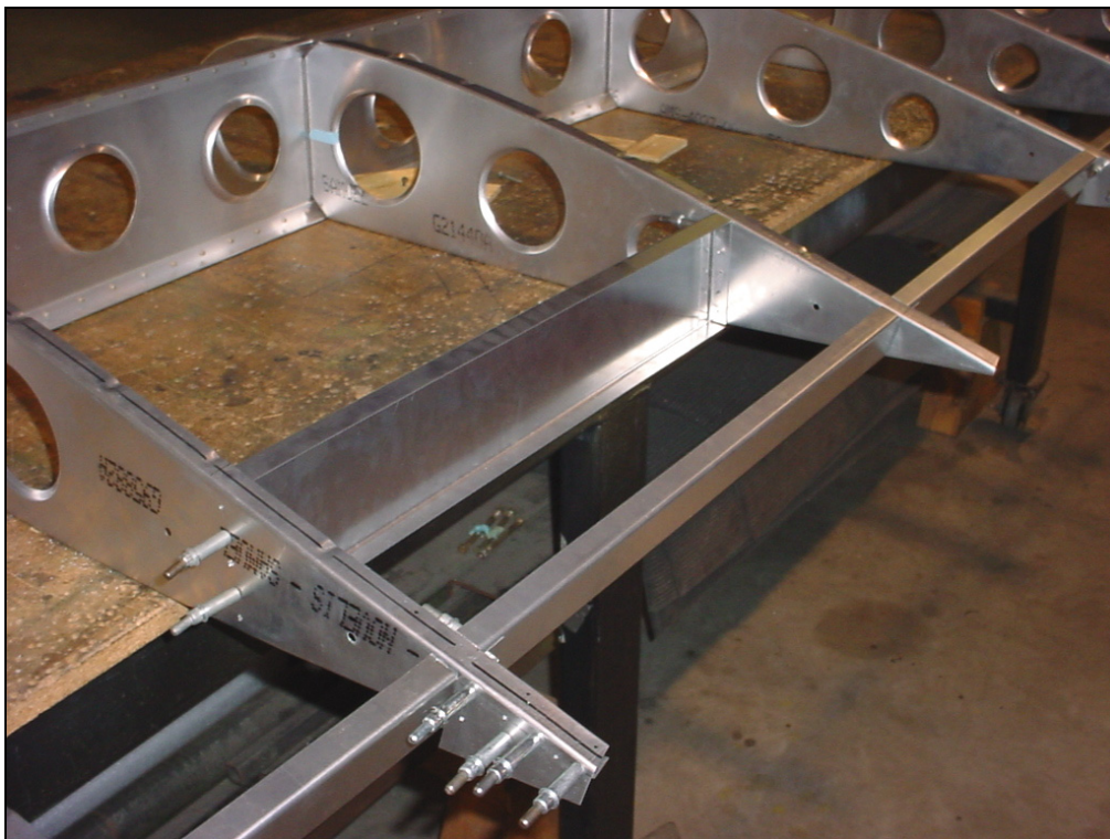
Clamp the extrusion to the rib flange.
