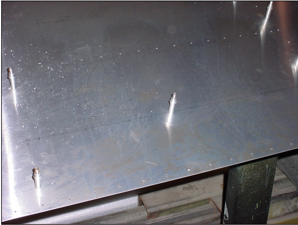
Drill and Cleco the rivet line through the wing tank channel.
