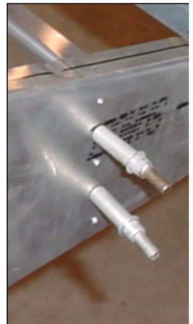
Drill and cleco.
