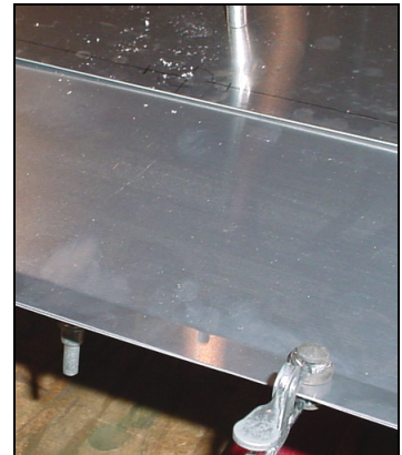
Clamp the trailing edges flush.
