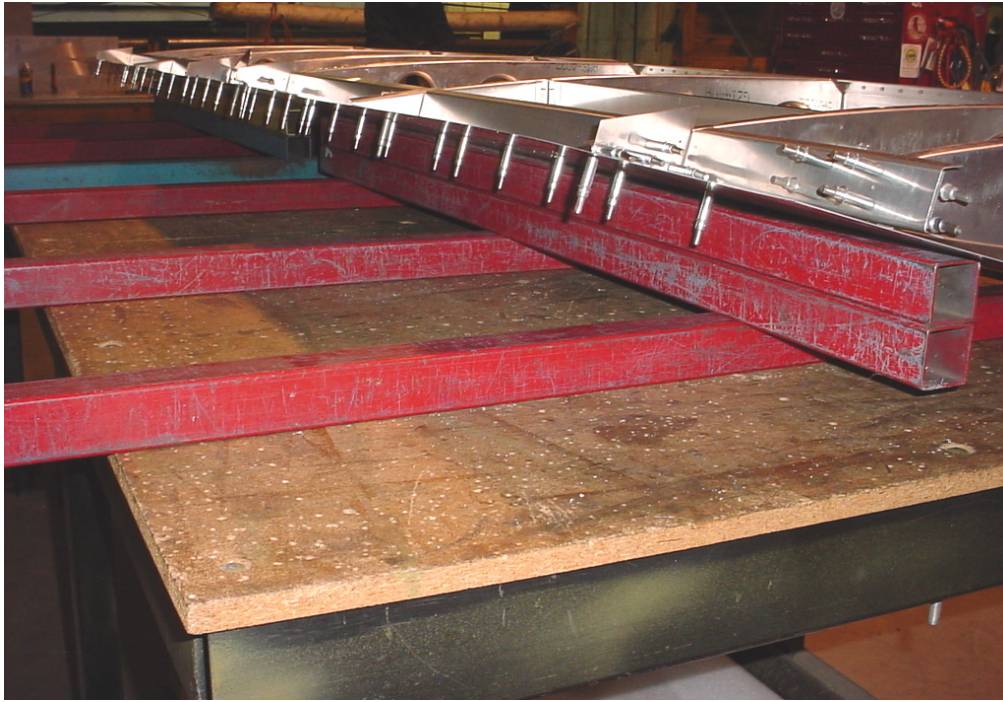
Supports beams under the rear of the wing . Adjust the position of the support beams to keep the spar vertical.
