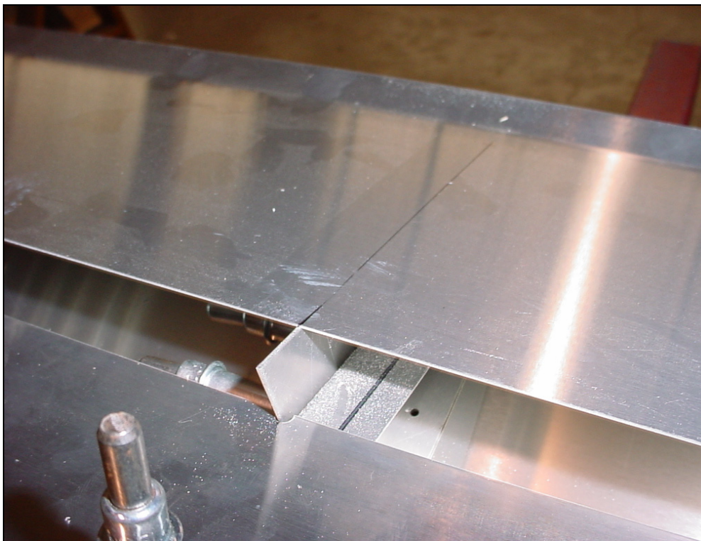
Location of the slots over the bracket.
