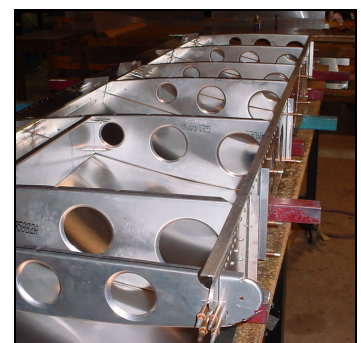
Mark the rivet line on the rib flanges and channels.
