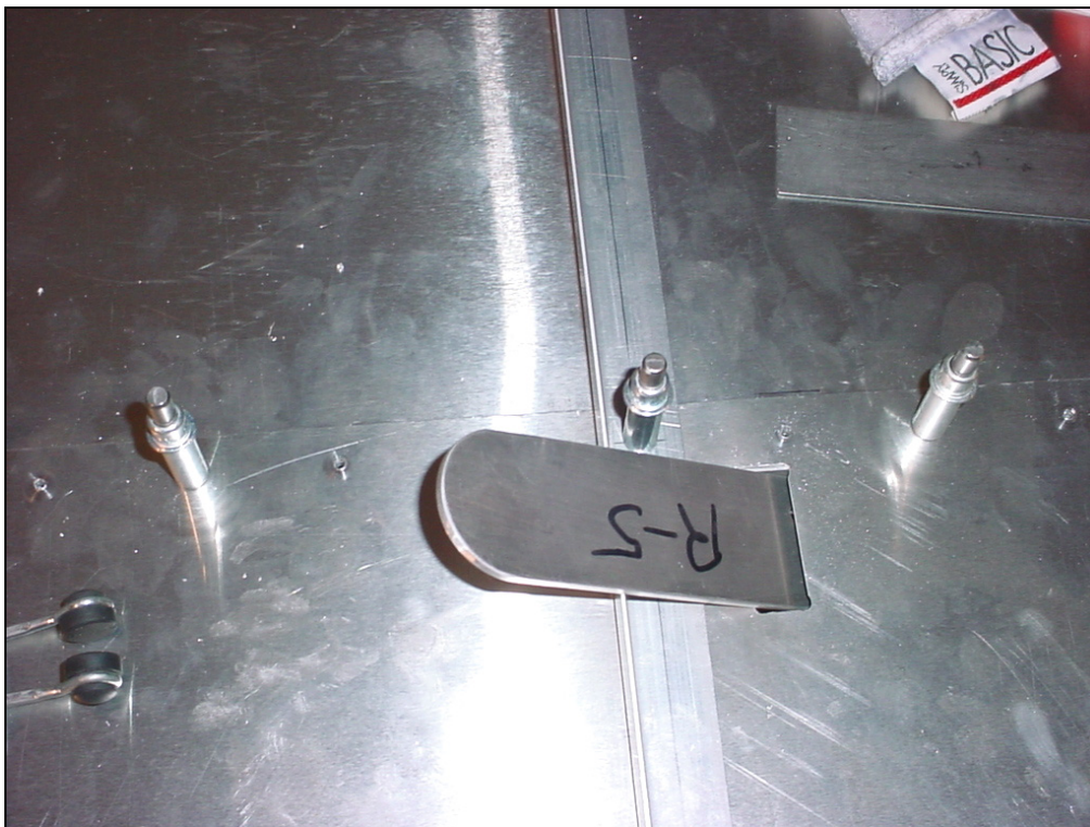
Mark the spar rivet line on the angle.
