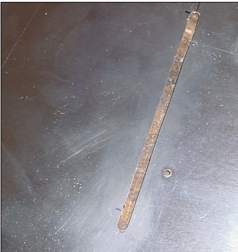
This is the finished slot after drilled and filed.
