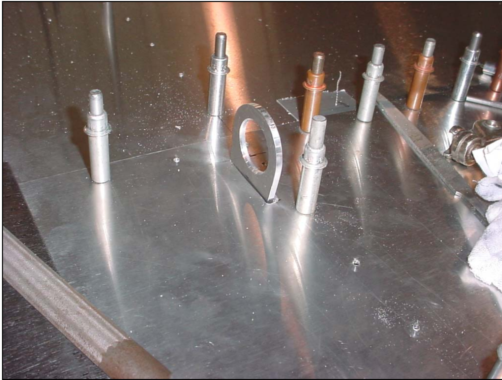
Tie down ring on the bottom side of the wing.
