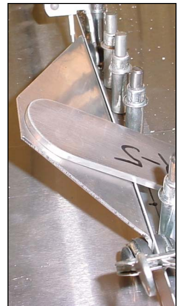
CLAMP: Clamp the sides to the L angle. CHECK: The end of the doubler is flush with the rounded end of the strut fitting
