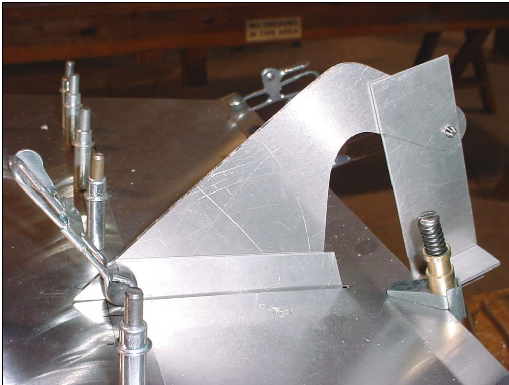
Position the template and arm on the wing and clamp the template to the trailing edge.
