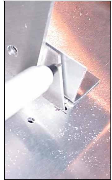
Aft detail: Trim L angle flush with the ends of the bracket 7V4-6
