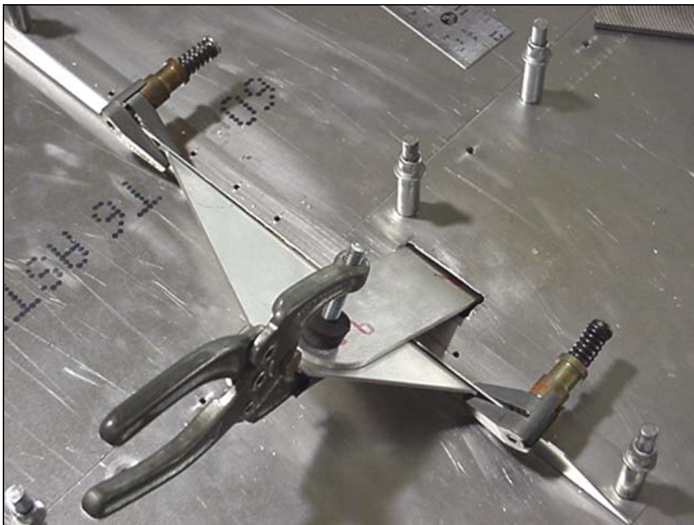
ORIENTATION: The short sloped side is towards the front. ReF. 7-V-8 Position 7V8-1SP under the upper strut fitting. CLAMP: Along the top, clamp to the strut fitting 7V2-5
