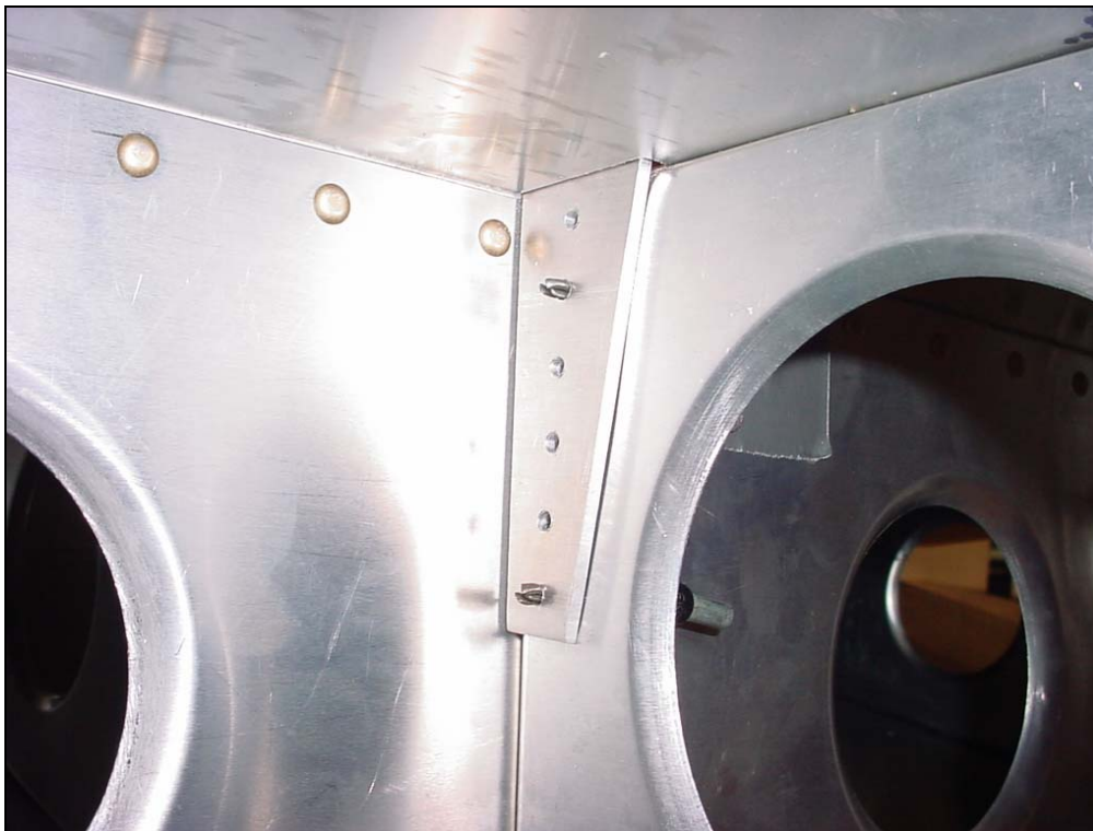
Drill and cleco 6 RIVETS A5 Ref. bottom diagram on drawing 7-V-8
