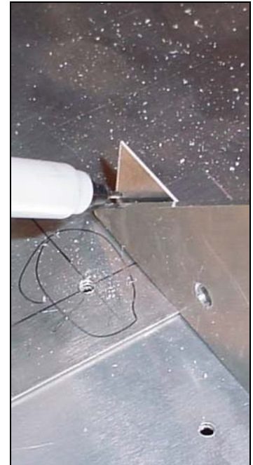
Detail of the front corner. Trimmed flush with the front edge of the arm 7V4-7
