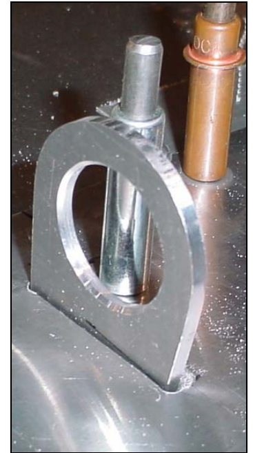
Detail of the 40mm reference line even with the skin
