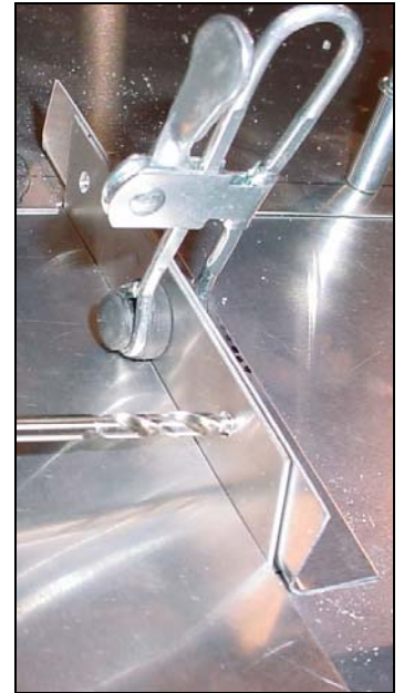
Back drill through the #20 in the bracket.
