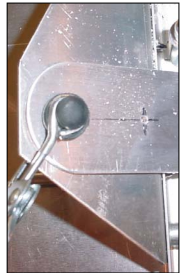
Before drilling, clamp the parts together.
