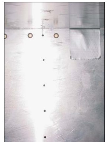
Check to make sure the location of the cutout is in front of the spar.
