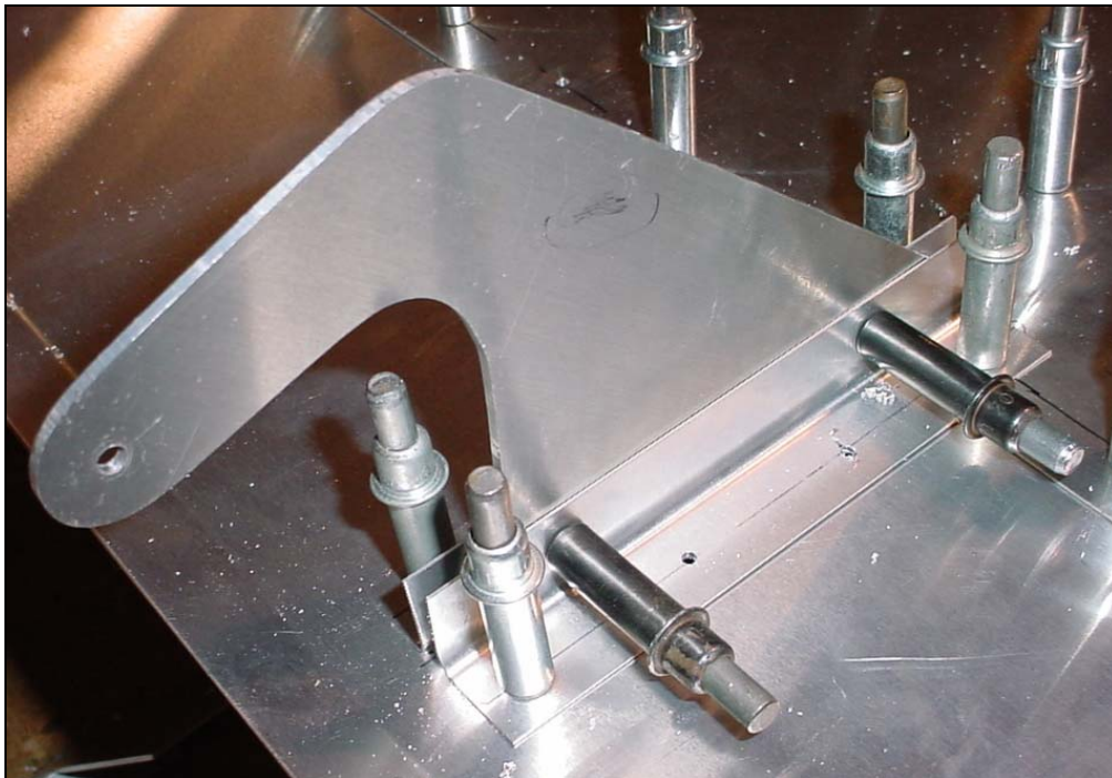
Cleco the arm and back drill through the second L angle.
