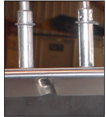
Detail: location of crimp between the rivets.
