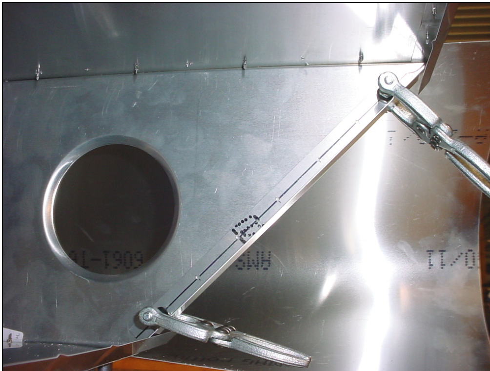
Clamp the L angle to the spar tip 7V3-3.
