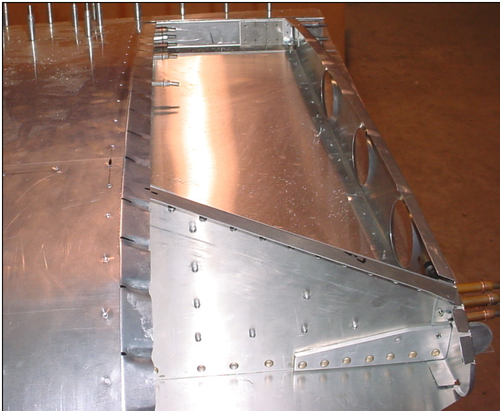
Check that the root angle and the root rib are both in line with the top flange of the spar root doubler 7V3-2SP
