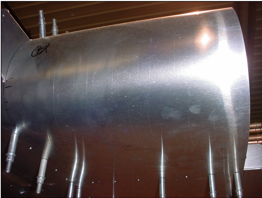
Top view of the leading edge (nose skin) 7V7-1. The leading edge skin will be trimmed to make the connection to the root nose rib.
