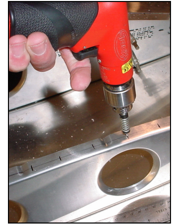
Pre-drill the rib flange with #40 pilot holes.
