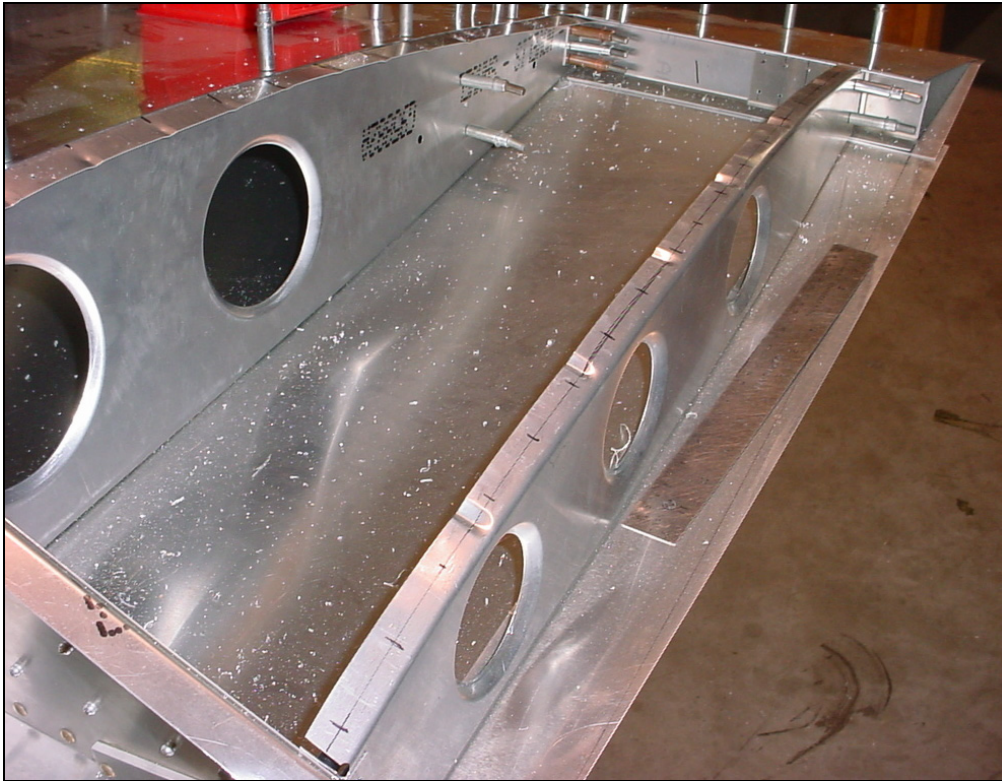
Pre-drill the rib flange with #40 pilot holes.
