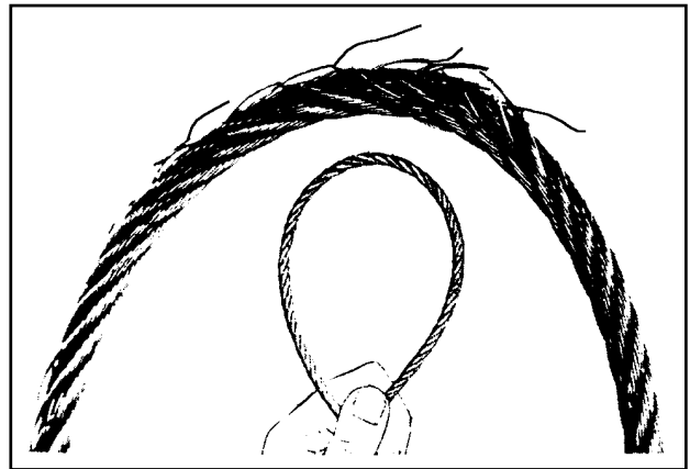
FIGURE 7-16. Cable inspection technique.
