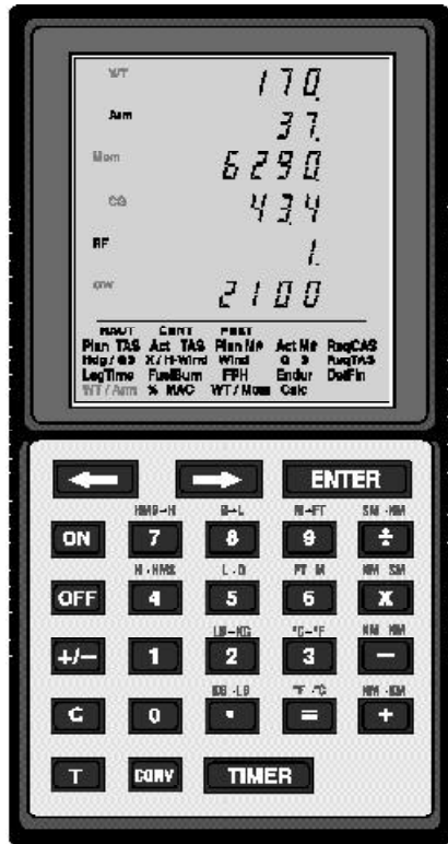
Figure 8-3. Dedicated electronic flight computers are programmed to solve weight and balance problems as well as flight problems.
