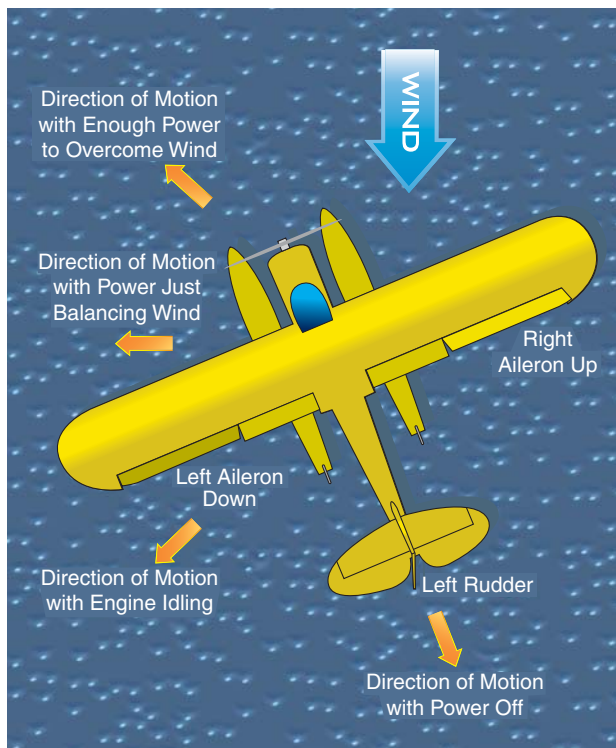
Figure 4-12. By balancing wind force and engine thrust, it is possible to sail sideways or diagonally forward. Of course, reversing the control positions from those illustrated permits the pilot to sail to the opposite side.
