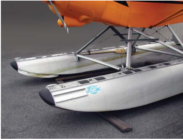
Figure 4-1. A preflight inspection with the seaplane on land provides an opportunity to thoroughly examine the floats below the waterline. Note the spray rail on the inboard chine of the far float in this photo.
