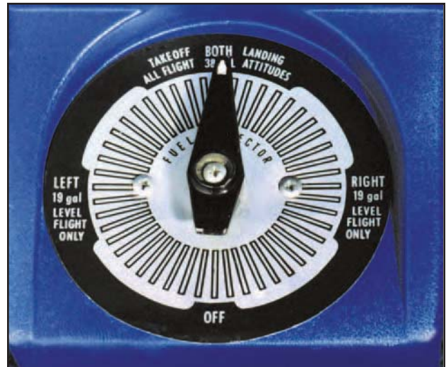
Figure 5-16. Fuel selector valve.
