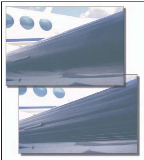
Figure 5-34. De-icing boots on the leading edge of the wing.
