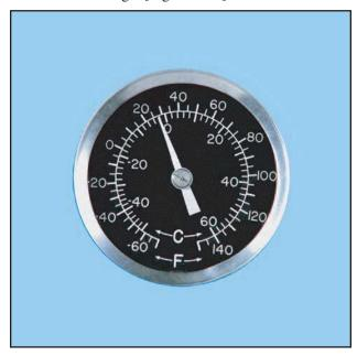
Figure 6-24. Outside air temperature gauge.
