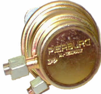
996 594 - 912 fuel pump with threaded fittings
