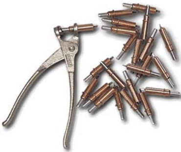
'Cleco' temporary fasteners
