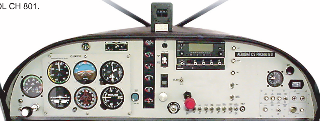
A typical STOL CH 801 Instrument Panel Layout
