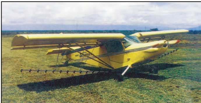
A custom STOL CH 701 taildragger equipped with low-volume ag spray system (South America).
