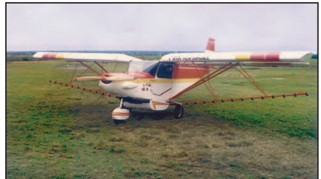
STOL CH 701 custom-configured with a low-volume ag spray system and a belly pod.
