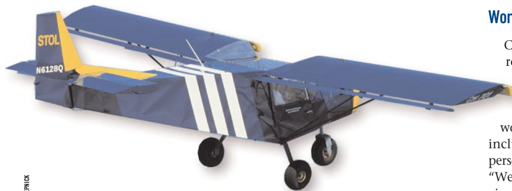
The most important feature of any STOL aircraft is its wing, which must have a high-lift coefficient to provide short takeoff and landing performance. Here you can easily see the leading edge slats, painted in yellow, on Roger Dunham's CH 701. At the back of the wing, full-span flaperons help to increase lift and provide good roll stability. Hoerner wingtips, a trademark of Heintz's designs, help keep airflow attached to the wing by maximizing the effective lift area while still minimizing the wingspan. To learn more about STOL design, read Heintz's "High-Lift Wing Design," at www.zenithair.com/stolch701/7-design-wing.html .
