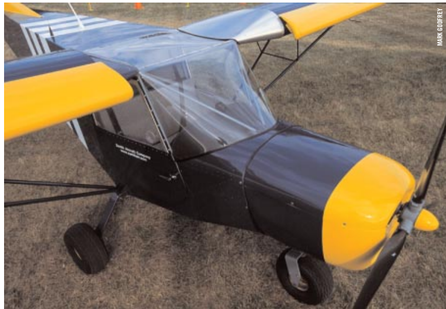
A full-cabin skylight and large windshield and side windows offer excellent visibility. Extra-wide tires provide for a sure grip on landing at airports or off-airport unimproved fields.
