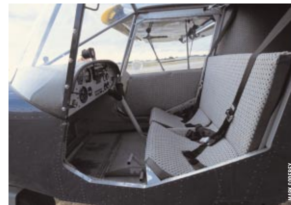
The CH 701's cabin is 41 inches wide at the shoulders. A baggage area behind the seats offers some in-cabin storage space. The aircraft's top-hinged doors make entry and exit from the aircraft easy, especially on floats.
