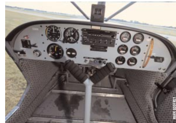
While Roger's 701 is a working "Sky Jeep," and shows a little wear on the cabin floor, it still provides a good look at the wide panel and distinctive Y-yoke common in Heintz-designed aircraft. Here's another scheme for outfitting your panel.
