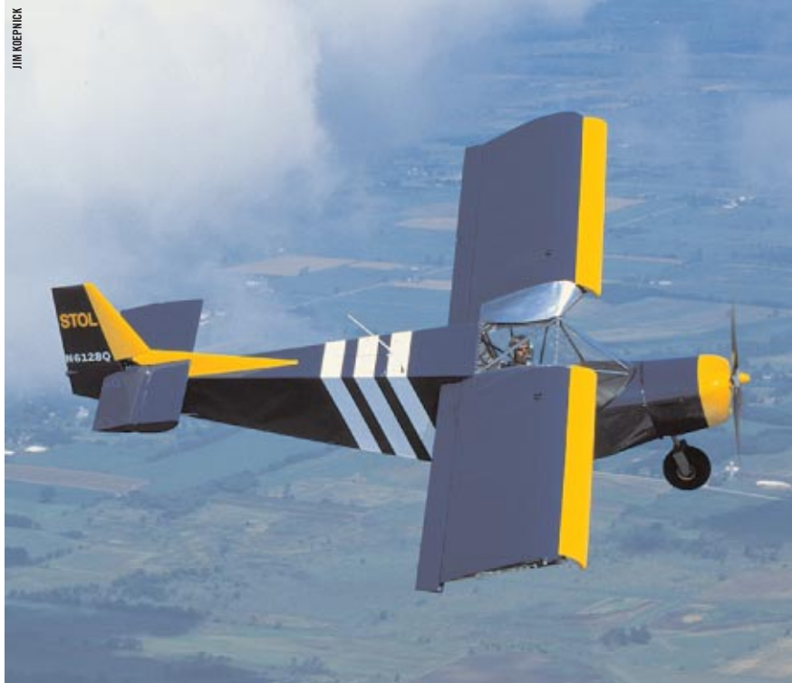
The most important feature of any STOL aircraft is its wing, which must have a high-lift coefficient to provide short takeoff and landing performance. Here you can easily see the leading edge slats, painted in yellow, on Roger Dunham's CH 701. At the back of the wing, full-span flaperons help to increase lift and provide good roll stability. Hoerner wingtips, a trademark of Heintz's designs, help keep airflow attached to the wing by maximizing the effective lift area while still minimizing the wingspan. To learn more about STOL design, read Heintz's "High-Lift Wing Design," at www.zenithair.com/stolch701/7-design-wing.html .
