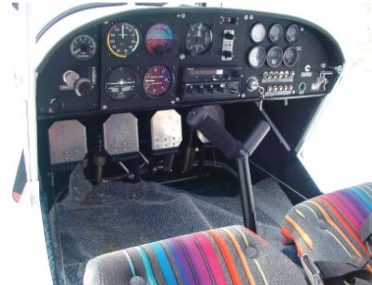
While Roger's 701 is a working "Sky Jeep," and shows a little wear on the cabin floor, it still provides a good look at the wide panel and distinctive Y-yoke common in Heintz-designed aircraft. Here's another scheme for outfitting your panel.
