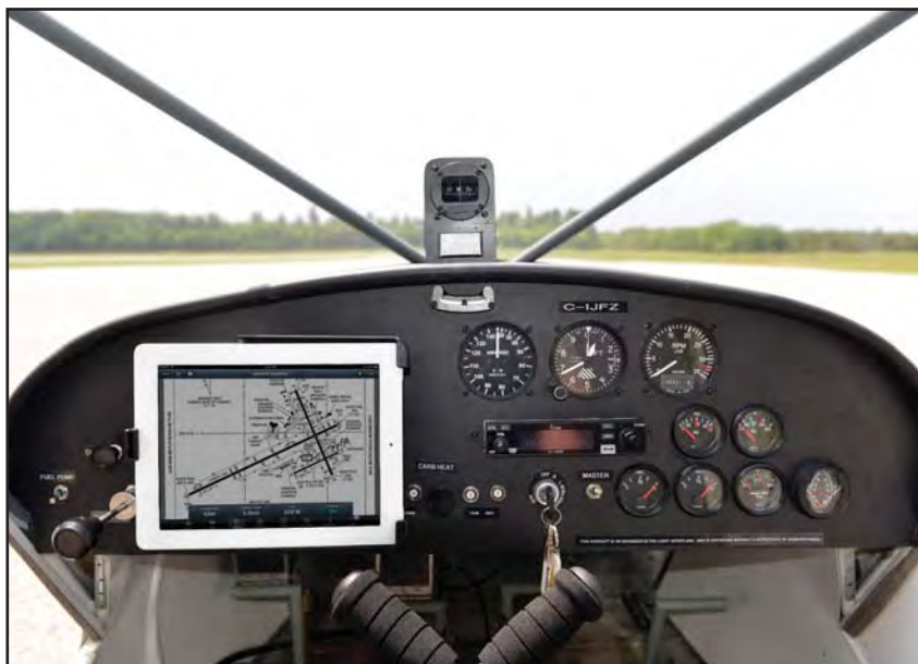
A CH 750 panel featuring a combination of “steam gauges” side-by-side with an iPad.
